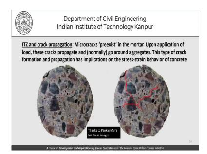
When it comes to crack propagation, it is very clear from the picture that I have been showing you all the time micro cracks pre-exist in the mortar. Upon application of load these cracks propagate and normally go around the aggregates. Now, I have already said that this going around the aggregate really means going through the ITZ. This type of crack formation and propagation has implications on the stress strain behaviour of concrete.
