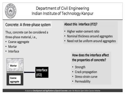
So, as far as our brief discussion today is concerned, we have talked of the concrete as a threephase material the coarse aggregate, mortar and interface and we have discussed how the ITZ affects the strength, crack propagation and the stress strain curve. The stress strain curve I have not discussed so much, I have just left it to you with a reference, I hope that would be good for you to have an understanding of that and you will be better off with reading.
