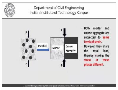
When it comes to parallel, both the mortar and coarse aggregate are subjected to the same level of strain. However, they share the total load thereby making the stresses in these phases different. So that is the kind of impact that the ITZ has on the strength of concrete.
