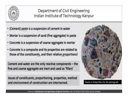
And, we had said that well as far as the basic model is concerned, we will talk of cement paste as a suspension of cement in water, mortar as a suspension of sand in paste and concrete as a suspension of coarse aggregate in mortar. So, with this understanding we move forward and said that concrete is a composite and its properties are related to those of its constituents and the relative proportions primarily.
