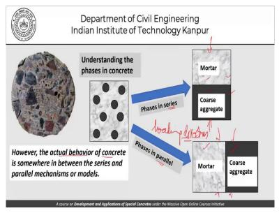
If we try to divide this discussion into phases part of it, we can talk of the phases in series. Now, what the series part of it will come in a minute, this is what it is so here we have mortar and coarse aggregate aligned like this, when it comes to parallel, we can talk of mortar and coarse aggregate align like this. The series and parallel is a nomenclature, which I am using in the light of or considering the loading direction.
