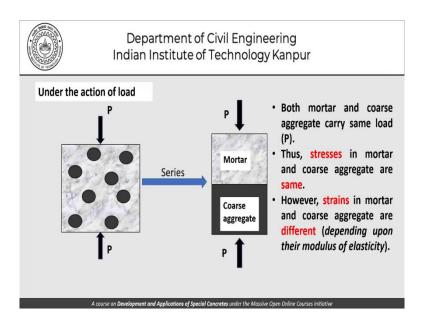
Having said that, the action under load as far as series is concerned is something like this both mortar and coarse aggregate carry the same load P. The stresses in water and the coarse aggregate are the same and the strains in mortar and coarse aggregate are different departing depending upon their modulus of elasticity and so on.
