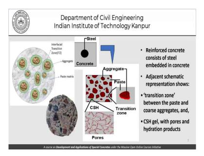
This is how, it goes carrying our understanding or our thought process further, reinforced concrete consists of steel embedded in concrete. So, this is the steel bar this is the concrete around it, this concrete looks like this, which we say that it can be modelled something like this. Now, what I have introduced here apart from the mortar and the coarse aggregate is this green zone around these aggregates and that is called the interfacial or intermediate transition zone that is the ITZ.
