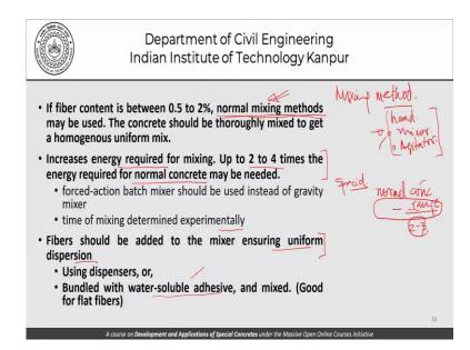
Now, coming to some transportation and construction issues, relating to fibre reinforced concrete, if the fibre content is between 0.5 and 2 percent, normal mixing methods may be used, Concrete should be thoroughly mixed to get a homogeneous uniform mix. What is a normal mixing method? Now only when you are starting to use special concretes and we are getting into the discussion here, for example, with fibre reinforced concrete, this idea of normal mixing method has been invoked.
