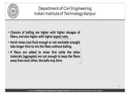
Chances of balling are higher with higher dosages of fibres are also higher with a higher aspect ratio. The aspect ratio means the length to diameter ratio of the fibres. Harsh mixes not fluid enough, not workable enough, take longer time to mix the fibres, without balling. If fibres are added to the mixer first, while the other materials are not enough to keep the fibres away from each other, again balls may form.
