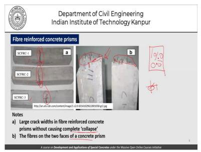
This picture here, before we get into properties of fresh concrete, a fresh fibre reinforced concrete, this picture here shows fibres is sticking out of the surface of concrete. So, this is something which we should visualize and connect to the previous discussion or the previous diagram where we try to show you, coarse aggregates here and mortar here and so this is the fibres that we are talking about.
