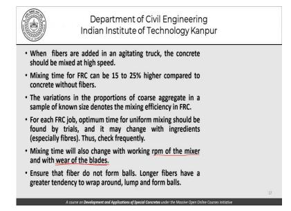
When fibres are added in an agitating truck, the concrete should be mixed at high speed. Mixing time for fibre reinforced concrete can be 15 to 25% higher compared to concrete without fibres. The variation in the proportions of coarse aggregate in a sample of known size denotes the mixing efficiency of fibre reinforced concrete. For each fibre reinforced concrete job, the optimum time for uniform mixing should be found by trials.
