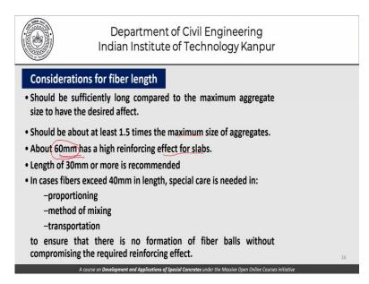
As far as considerations for the length of fibres is concerned, they should be sufficiently long compared to the maximum size of the aggregate to have the desired effect. Of course, there are applications in which shorter fibres are also used. They should be at least 1.5 times the maximum size of aggregates but I just mentioned that there are applications where this rule need not be followed. We could use shorter fibres about 60 mm fibre lengths has a high reinforcing effect for slabs.
