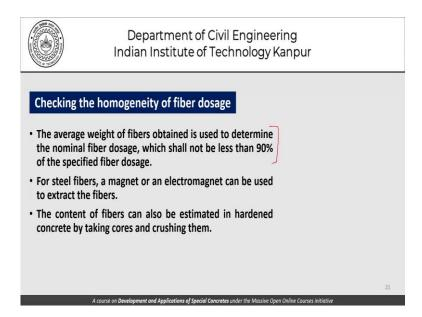
The average weight of fibres obtained is used to determine the nominal fibre dosage which should be not less than 90 percent of the specified fibre dosage. So, obviously once we do this kind of sampling, it need not meet the exact number that we had thought of. So, if we had put in two percent in a given sample it can be plus or minus a little bit and that is what the codes will tell us that it should not be less than ninety percent of the specified dosage.
