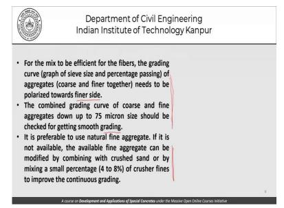
For the mix to be efficient for the fibres, the grading curve, the graph of the sieve size and percentage passing of aggregates, coarser and finer together, needs to be polarized towards the finer side. The combined grading curve of coarse and fine aggregates down up to 75 micron size should be checked for getting a smooth grading. Its suggesting is that as far as normal concrete is concerned or compared to what normal concrete demands are the grading
