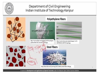
Now, this is again a reiteration of the type of fibres that we use steel, polyethylene, maybe aramid glass and so on. Now, the extent of modification in the properties of the concrete would depend on the fibre volume and the fibre characteristics. So, obviously whether it is the properties of fresh concrete or whether it is the properties of hardened concrete, this simple thumb rule will still operate.
