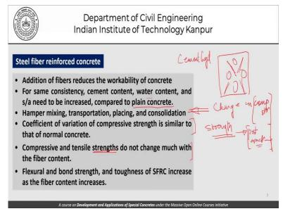
Moving forward the compressive and tensile strengths do not change with the fibre content this is especially true in low volume addition of fibres. So, long as the fibre addition does not exceed say two percent or one at least one and a half to two percent, we do not expect much change in the compressive or tensile strength as such. Strength means the maximum load that it can take.
