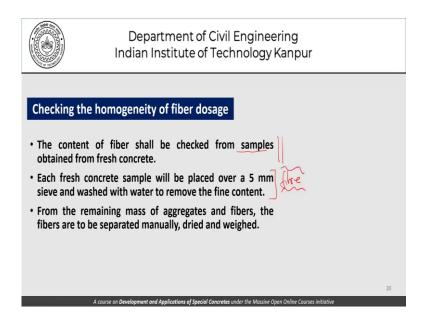
When it comes to checking the homogeneity of fibre dosage, it is very important to ensure the fibre dosage that we have added is indeed, uniformly spread across the entire concrete and for that the content of fibre shall be checked from samples obtained from fresh concrete. So, unlike coarse aggregates, where we do not do such tests unless we are looking for segregation for fibres it is important that such a test is carried out to ensure that the concrete has fibres in each location.
