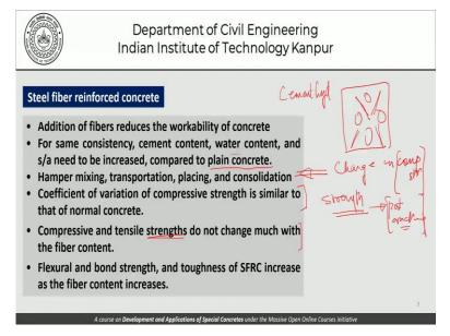
Now, as far as steel fibre reinforced concrete is concerned and this discussion is true with other fibres as well, the addition of fibres reduces the workability of concrete. So, you can very well imagine that if we have a matrix like we had, with coarse aggregate here, the rest of it being mortar, if I put fibres here, it will reduce the workability of the mortar phase and consequently of the concrete phase.
