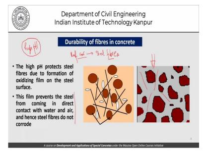
This is the picture which I had shared with you last time and I had left you with an assignment as to why steel fibres do not corrode or what is the kind of issues that we must be careful about as far as durability of the fibres within the concrete matrix is concerned. We had highlighted the fact that it is a high pH environment and therefore particularly glass fibres were mentioned to the extent that there could be durability issues with glass when it is exposed to high ph environment.
