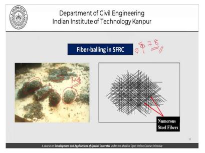
This is what is the concept of balling if we do not mix or disperse the fibres carefully they may tend to accumulate at one place and form balls. So, we should be very careful that the fibres do not form such kind of balls within the concrete. One should remember that the specific gravity of steel is 7.8 and this is much, much heavier than all the constituents as far as concrete is concerned.
