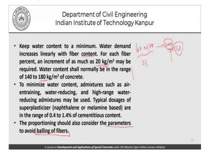
We need to keep the water content to minimum, yes but the water demand increases linearly with fibre content, so the more the fibre, more water you need for a given level of workability or consistency. And for each fibre percentage an increment of as much as 20 kgs may be required and water content shall normally be in the range of 140 to 180. This is just a range; this number is again just a indicative number.
