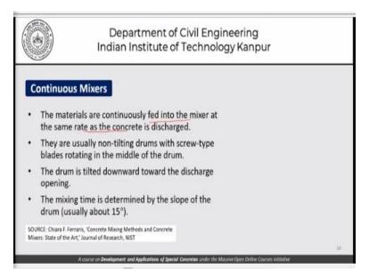
Now coming to continuous mixers, in this the material is continuously fed into the mixer at the same rate as the concrete is discharged. This balance of the rate of concrete discharge and the rate of feed into the mixer has obviously to be maintained. In order that the concrete of a certain consistency as far as the constitution is concerned can still be obtained. Now they are usually non tilting drums with screw type blades rotating in the middle of the drum.
