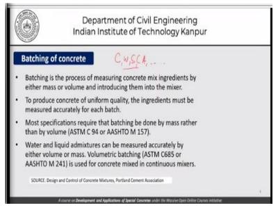
Batching of concrete is the process of measuring concrete mix ingredients by either mass or volume and introducing them to the mixer. We have talked about the mix ingredients when we are talking about proportioning. And we know that we need to proportion cement, water sand and coarse aggregate at least, and possibly other things like chemical admixtures or mineral admixtures and we have a specific mass associated with them.
