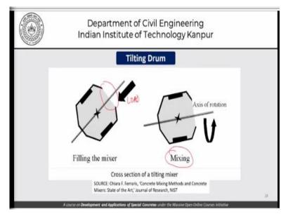
Here is a schematic representation of a tilting drum mixer with the cross section of this mixer shown here. So, we have this opening here which is used for the loading the mixer as well as discharging it, so it is at this position that we load the mixer. Then we make it basically horizontal or just half horizontal rotate the mixer and mix the concrete. So, this is the mixing process that is going on as far as this mixer is concerned.
