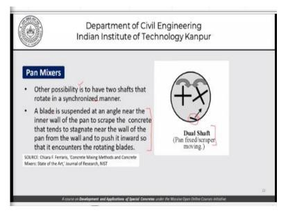
This one is another type of a pan mixer where we have a dual shaft that is we have two shafts. The other possibility as is listed here is to have two shafts that rotate in a synchronized manner. A blade is suspended at an angle near the inner wall of the pan to scrape the concrete that tends to stagnate near the walls of the pan from the wall and to push it inwards, so that it encounters the rotating plates.
