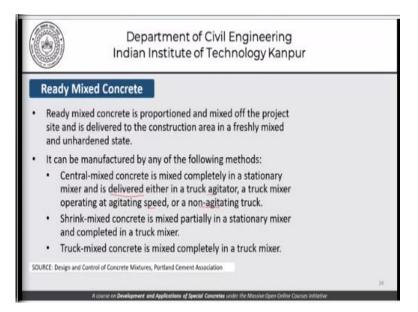
As far as the ready mixed concrete is concerned, this concrete is proportioned and mixed off the project site and is delivered to the construction area in a freshly mixed and unhardened state. That is something which we need to ensure that the concrete is delivered to the construction site from the ready mixed concrete plant, it should be freshly mixed and obviously unhardened. It can be manufactured by any one of the following methods.
