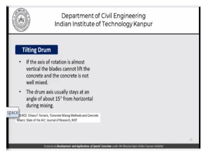
If the axis of rotation is almost vertical the blades cannot lift the concrete and the concrete is not mixed well. The drum axis usually stays at an angle of about 15 degrees from the horizontal during mixing.
