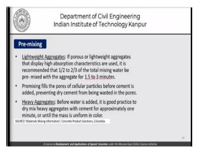
As far as pre-mixing is concerned, that is something which we shall remove all this. Now coming to pre-mixing as far as lightweight aggregates are concerned, they need to be pre-mixed. If porous or lightweight aggregates that display high absorption characteristics are used, it is recommended that half to two-thirds of the total mixing water be pre-mixed with the aggregates for about one and a half to 3 minutes.
