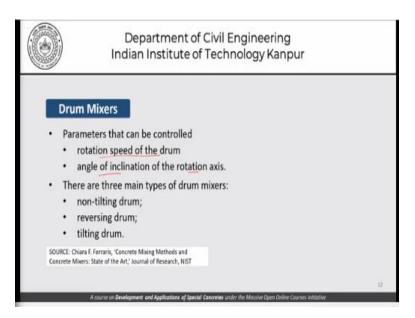
Continuing with our discussion on drum mixers, the parameters that can be controlled is the rotation speed of the drum and the angle of inclination of the rotation axis if any. There are three main types of drum mixers the non-tilting type, the reversing drum and the tilting drum.
