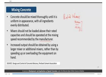
And we try to come to the discussion on mixing concrete, the concrete should obviously be mixed thoroughly until it is uniform in appearance with all it is ingredients uniformly distributed, that is the essence of the mixing process. The mixers should not be loaded above their rated capacities and should be operated at the mixing speed recommended by the manufacturer. So, there is manufacturer involved who tells the operator as to what is the mixing speed that is recommended.
