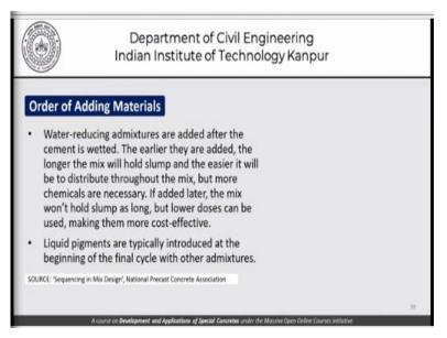
Water reducing admixtures on the other hand are added after the cement is wetted. The earlier they are added the longer the mix will hold the slump and the easier it will be to distribute throughout the mix but more chemicals will be necessary. If added later the mix will not hold slump as long but lower doses can be used making them more cost effective. Liquid pigments are typically introduced at the beginning of the final cycle along with other admixtures.
