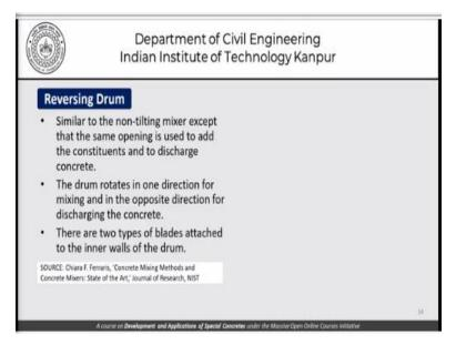
As far as a reversing drum mixer is concerned, it is similar to the non tilting mixer except for the fact that the same opening is used to add the constituents and to discharge the concrete. The drum rotates in one direction for mixing and the opposite direction for discharging of concrete. There are two types of blades attached to the inner walls of the drum as far as a reversing drum is concerned.
