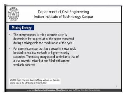
Let us go back to our discussion on the mixing energy. So, the energy needed to mix a concrete batch is determined by the product of the power consumed during a mixing cycle and the duration of the cycle. So, it is really the power times the duration that gives you the energy. As far as research is concerned, you could be talking in terms of the energy required per cubic meter of concrete.
