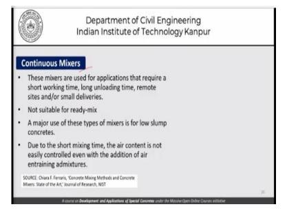
Continuing our discussion about continuous mixers, these mixers are used for applications that require a short working time, long unloading times, remote sites and or small deliveries. They are not particularly suitable for large volumes of concrete to be mixed or delivered. They are not suitable for ready mixed operations and a major use of these types of mixers is for low slump concretes, high slump concretes are difficult to get out of these continuous mixers.
