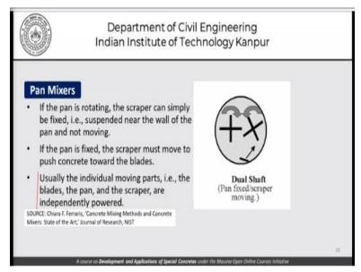
Now continuing our discussion of pan mixers, if the pan is rotating, the scraper can simply be fixed. That is, it can be suspended near the wall of the pan and not moving, if the pan is fixed however the scraper must move to push the concrete towards the blades. And usually, the individual moving part that is the plates, the pan and the scraper are independently powered, that is something which we must bear in mind.
