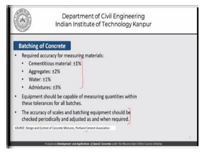
And things with our discussion of batching some of the benchmarks which are available to us are the required accuracy for measuring materials could be 1% for cementitious materials, 2% for aggregates, 1% for water and maybe 3% for admixtures. These numbers will obviously be different for different specifications and this is the source that we are using here. So, I will encourage you to take up some other source of information.
