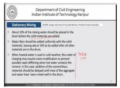
Moving forward with stationary mixing about 10% of the mixing water should be placed in the drum before solid materials are added. So, this is a characteristic or this is a suggestion or a guideline as far as stationary mixing is concerned. That is 10% of the mixing water should be placed in the drum before solid materials are added. Water should then be added uniformly with the solid materials leaving about 10% to be added after all the other material is in the drum.
