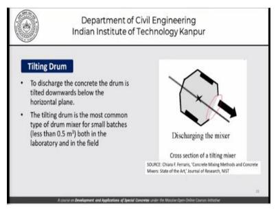
And finally, we tilt the drum, in this direction that is shown for discharging the concrete from the mixer. So, it is the same opening being used for loading as well as discharging the concrete. So, to discharge the concrete the drum is tilted downwards below the horizontal plane. The tilting drum is most common type of mixer for a small batches less than about 0.5 cubic meters, which is about 500 liters of concrete both in the laboratory and in the field.
