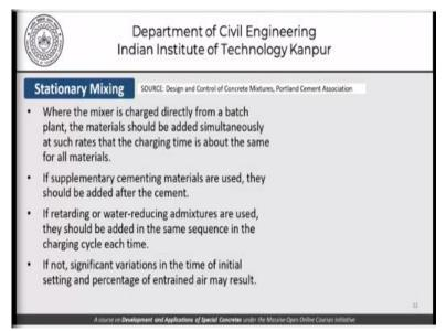
Where the mixer is charged directly from a batching plant, the material should be added simultaneously at such rates that the charging time is about the same for all the materials. And if supplementary cementing materials are used, they should be added after the cement. If retarding or water reducing admixtures are used, they should be added in the same sequence in the charging cycle each time.
