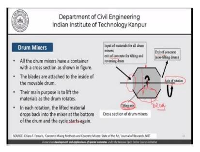
As far as drum mixes are concerned, this is a schematic representation of these mixers. We said that the axis of rotation is largely horizontal or slightly inclined. And we have input of materials for all drum mixers at one side here. And the exit of the concrete for tilting or reversing the drum at this end, sometimes in a non-tilting drum we have the exit of concrete on the other side. Whereas this largely remains the tilting axis and this axis is the tilting axis.
