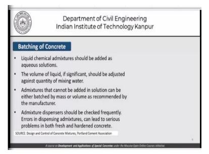
Liquid admixtures or liquid chemical admixture should be added as aqueous solutions. We can dilute them by using water which needs to be adjusted again with respect to the amount of total mixing water that we use the volume of liquid, if significance should be adjusted against the quantity of mixing water. Admixtures that cannot be added in solution can be batched by mass or volume as recommended by the manufacturer.
