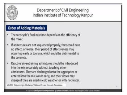
The wet cycle's final mixing time depends on the efficiency and the power of the mixer and also the kind of concrete being used and the volume. If admixtures are not sequenced properly, they could have no effect or worse their period of effectiveness may occur too early or too late which could obviously be detrimental as far as properties of concrete are concerned. Reactive air entraining admixture should be introduced into the mix separately without touching other admixtures.
