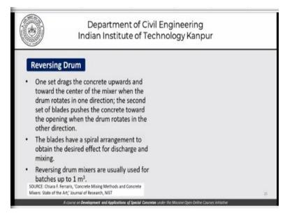
One set of blades drags the concrete upwards and towards the center of the mixer when the drum rotates in one direction. And the second set of blades pushes the concrete towards the opening when the drum rotates in the other direction at the time of discharge. The blades have a spiral
