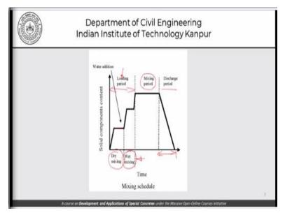
This picture shows a rough schematic diagram of the mixing schedule or the steps in the mixing process. So, we can see that these are the solid components that are being added gradually, there is a stage of dry mixing of concrete, there is wet mixing of concrete. Then we have the mixing period, this period overall is called the loading period. Then the mixing period and this is the discharge.
