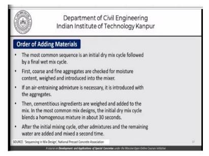
Coming back to our discussion on the order of adding materials the most common sequence is an initial dry mix cycle followed by a final wet mix cycle. First the coarse and fine aggregates are checked for moisture content, weighed and introduced into the mixer. If an air entraining admixture is necessary, it is introduced with the aggregates. Then cementitious ingredients are weighed and added to the mix in the most common mix designs.
