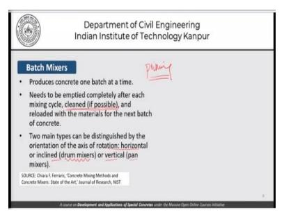
As far as batch mixers are concerned, as the name suggests they produce one batch of concrete at a time. That is if it is a 2 cubic meter batch mixer, you put the ingredients there for 2 cubic meters mix it and discharge it which gives us the 2 cubic meters of concrete. And then we add the next batch, so that is what is the principle of a batch mixer, it produces one batch at a time. A batch mixer needs to be completely emptied after each mixing cycle.
