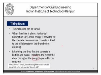
Coming to the tilting drum, the angle of inclination can be varied and when the drum is almost horizontal that is having no inclination 0 degrees. More energy is provided to the concrete because more concrete is lifted to the full diameter of the drum before dropping. And it is during the drop that the concrete is actually knitted and mixed. Therefore, the higher the drop, the higher the energy imparted to the concrete.
