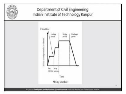
Once again, I show you this schematic representation of the mixing process. The dry mixing, the wet mixing, the real mixing period and the discharge on a schematic diagram.
