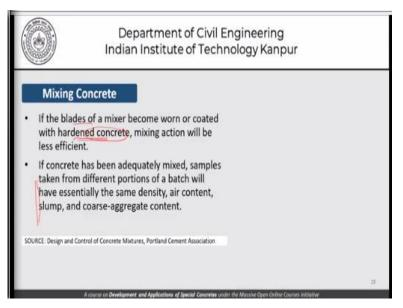
If the blades of a mixer become worn or coated with hardened concrete, the mixing action will be inefficient. So, we have to make sure that the blades of the mixture are not worn out and they are not coated with hardened concrete. Now in order to ensure that they are not coated with hardened concrete it is important to ensure that at the end of a mixing operation, the mixers are thoroughly washed.
