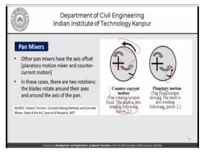
Continue our discussion with pan mixers, another type of pan mixers is one where the axis offset, that is planetary motion mixer and the counter motion mixer as is shown here. So, in this case we have a planetary motion mixer and a counter current motion. In this case in the counter current motion the pan rotating, scraper is fixed and the shaft is also rotating following this arrow 2, so this shaft rotates following this arrow here.
