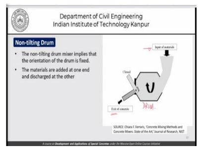
So, coming to the first part of our discussion the non tilting drum mixers, as we can see here this is the drum and we have the input of materials at one end of the drum and the exit of concrete at the other end. So, the non-tilting drum mixer implies that the orientation of the drum is essentially fixed. The material is added at one end of the drum and is discharged at the other.
