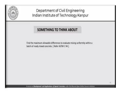
What is the maximum allowable difference to evaluate mixing uniformity within a batch of ready mixed concrete plant? Obviously, we understand from statistics that no matter how hard we try, we cannot get the same quality, exactly same quality from one batch to another. The only thing is there has to be a control on the extent of variation, and what is the level of variation that is allowed as far as different batches are concerned.
