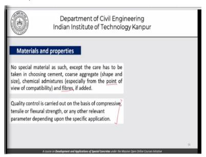
As far as the materials and properties are concerned for the shotcrete, no special material as such is required except care has to be taken in choosing the cement coarse aggregates in terms of shape and size. Chemical admixtures from the point of view of compatibility and also what we expect the chemical admixtures to do whether we are talking in terms of water reduction, whether we are talking in terms of acceleration and of course if we want to add fibres.
