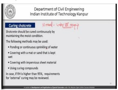
As far as curing of concrete is concerned, like any other concrete it needs to be cured, charcoal should be cured continuously by maintaining the moist condition. The following methods may be used, ponding or continuous sprinkling of water if possible, covering with a mat or sand that is kept wet, covering with an impervious sheet material using curing compounds. And in case the relative humidity is higher than 95% requirements for external curing may be reviewed.
