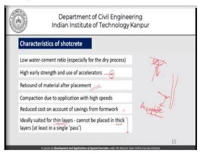
So, as far as the characteristics of shotcrete is concerned, low water cement ratio especially for the dry mix, high early strength and use of accelerators. This is something which is very important because the more time the concrete takes to set, the more is the real danger for the concrete falling off or moving away from where it is supposed to be or moving away from the state of placement.
