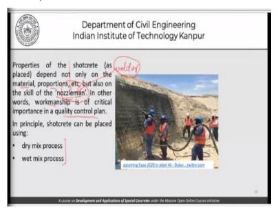
We should remember that the properties of shotcrete as placed depend not only on the material that we use or the proportions. But also, on the skill of the nozzleman, that is the workmanship is of critical importance in a quality control plan dealing with shotcrete. It is much more important here to have a trained or a qualified nozzle man than in normal concrete. I am leaving it to you to
