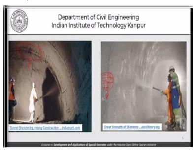
Before we start a discussion on the properties of shotcrete and the material used and so on, I will quickly go through some pictures to show you what the operation is and how it looks like when the concreting is being done in that manner. So, here we have one application where you can see shotcreting being carried out for tunnel linings. And you can see that the lining thickness need not be deposited in a single layer.
