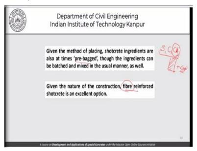
Moving forward given the method of placing, shotcrete ingredients are also at times pre-banged though the ingredients can be batched and mixed in the usual manner as well. Pre-bagging means we have a bag of pre-mixed shotcrete material, that is sand, cement and whatever coarse aggregate is required. That can all be put together in a certain proportion and sold in a pre-mixed bag.
