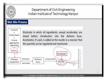
As against this in the wet mix process the cement, sand and coarse aggregate which is optional as I said before and water all of the concrete ingredients are added to the delivery equipment and the concrete is shot into the placing surface straightaway. So, what the difference is that here the entire delivery is for a wet concrete, wet to the extent that water has been pre-added to the mix much like any normal concrete.
