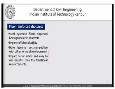
As far as fibre reinforced shotcrete is concerned, yes, the steel synthetic fibres dispersed homogeneously in shotcrete. We have talked about different types of fibres when we are talking about fibre reinforced concrete. And this is one application where fibre reinforced concrete can be used in repair works for example. Impart sufficient ductility that is the normal expectation from fibre reinforced concrete.
