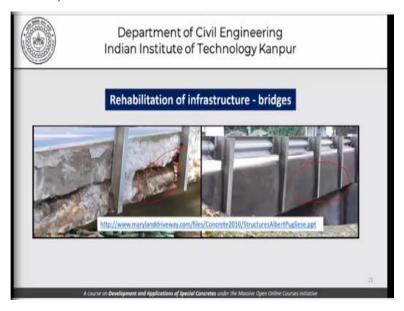
And then of course we have the rehabilitation of infrastructure may be bridges, where we can see this kind of deterioration. And this is the picture which we have after a deposit of shotcreting, not necessarily on this surface alone. But after the loose concrete and everything has been removed from here maybe additional reinforcement has been placed in position and then carrying out the shotcreting operation.
