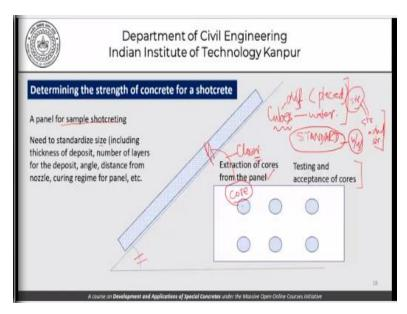
This slide is something which we have seen before. As far as determination of the strength of concrete under the shotcrete operation is concerned. There could be a mechanism by which we have a panel which is used to create the sample, which can then be used to extract coarse and we have testing and acceptance standards which are determined or which are laid out for accepting the shotcrete on the basis of strength.
