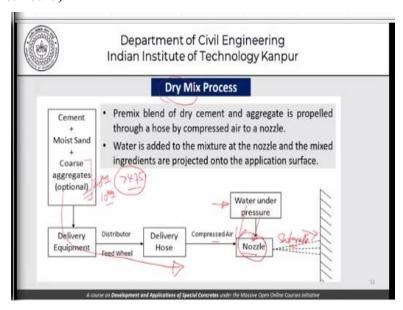
Now as far as the dry mix process is concerned, what happens is with cement, moist sand and coarse aggregate which is optional? Of course, in the context of shotcreting the coarse aggregate does not necessarily have to be 20 mm aggregate. Anything more than 4.75 mm qualifies as coarse aggregate and therefore we will have a lot of examples of shotcrete where only up to 10 mm kind of aggregates are used.
