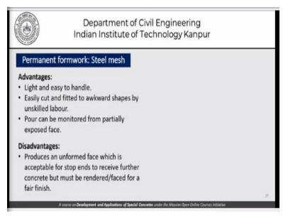
So, as far as the advantages of using this steel mesh formwork as a permanent formwork is that it is. Light and easy to handle, easily cut and fitted to awkward shapes; by practically unskilled labour. The pour can be monitored from partially exposed surfaces; we are talking of the pour of concrete. And the disadvantages of course are it produces an unformed phase which is acceptable for stop ends to receive further concrete what must be rendered or faced for a fair finish.
