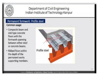
When it comes to permanent formwork with profile steel, the picture here shows how profile steel which is this part can be used to become a part of this slab kind of construction which is being done on top of this. And this formwork of course is not to be removed and steel reinforcement which is shown here can be a part of the normal placing. So, we have this formwork which we do not have to bother to remove.
