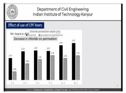
The last test I guess which was carried out was the decrease in the chloride ion permeation. And here we found that the chloride depth being measured in centimeters using a standard test was again much lower in the case of concretes with CPF liners. So, this study essentially established the importance or the effectiveness of using a CPF liner. If the client so permits, if the situations so demands and of course the economics of the CPF liners has to be worked out on a case-to-case basis.
