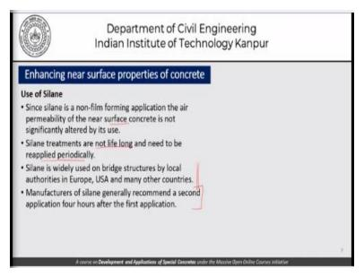
Since silane is a non-film forming application, the air permeability of the near surface concrete is not significantly altered by it is use. This treatment therefore is not life-long and needs to be reapplied periodically. Silane is widely used in bridge structures by local authorities in Europe, U.S and so many other countries. And I would encourage you to look at some literature which describes the use of silane in these structures in these countries.
