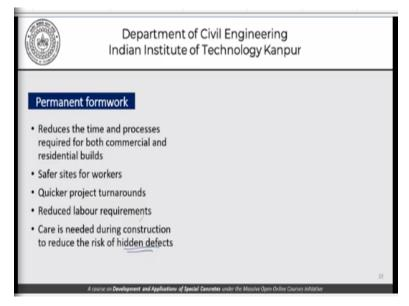
Reduces the time and processes required for both commercial and residential buildings, safer sites for workers, quicker project turnarounds, reduces labour requirement. And care of course needs to be taken during construction to reduce the risk of hidden defects. So, here we are talking of a situation or a construction method where the entire member is not precast, the precast construction the entire member would be precast.
