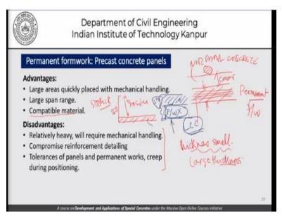
And the advantages of using this kind of formwork could be large areas could be quickly placed with mechanical handling. The formwork placement is much easier, large span ranges could be easily covered and the material is compatible. So, we do not have to bother about material compatibility because on both sides we have essentially cementitious mixes. Also, we can surely control the permeability of my permanent formwork by using special concretes.
