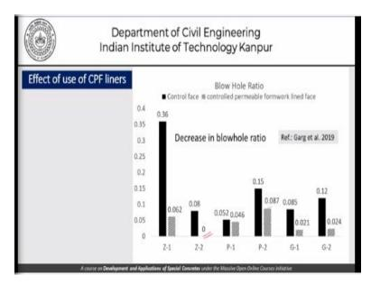
As we can see here the blowhole ratio is much lower in the case of CPF liners in fact it is 0 here. And this is yet another piece of evidence to show how the CPF liners can be very effective in improving the properties of the near surface concrete.
