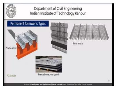
So, we have some examples of permanent formwork given here. This one is profile steel; this is a steel mesh and then of course there are precast concrete panels. So, these panels are the easiest to understand as far as permanent formwork is concerned. So, these panels become formworks and the concrete is cast on the inside of this panel. Similarly, the concrete is cast on the inside of this profile steel; we will see that in a minute.
