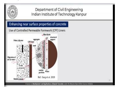
This is a diagrammatic representation of a control permeable formwork or a CPF liner. And we can see this reinforcement here, this is the CPF liner and fresh concrete being vibrated leads to the migration of air and water as shown here. Cement particles accumulating here and air and water being brought into this region and being taken off. So, this fabric essentially acts as a filter and drain, and this of course is the regular formwork that we are using.
