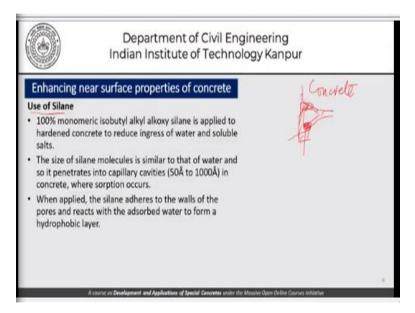
Now how do we go about addressing this problem? One way to address this issue of enhancing the near surface properties of concrete is by use of silane. 100% monomeric isobutyl alkyl alkoxy silane is applied to the hardened concrete to reduce the ingress of water and soluble salts. So, basically if we try to draw a schematic sketch and say that this is what my pores in the near surface region are.
