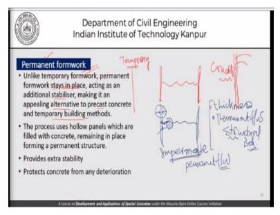
There is this concept of permanent formwork. Now what is permanent formwork? We have to view this against the temporary formwork which we normally use as far as concrete construction is concerned. So, let me reiterate that as far as concrete construction is concerned, we use a formwork, cast the concrete against that and then once it has hardened and so on, we remove the formwork, and we use it somewhere else.
