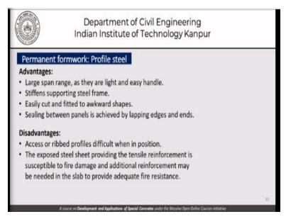
The advantages of using profile steel as permanent formwork are listed here. Large span range, they are light and easy to handle, stiffens the supporting steel frame, easily cut and fitted to awkward shapes, sealing between panel is achieved by lapping and edging the ends. There are disadvantages as well; there are always two sides to the coin access or ribbed profiles difficult when in position.
