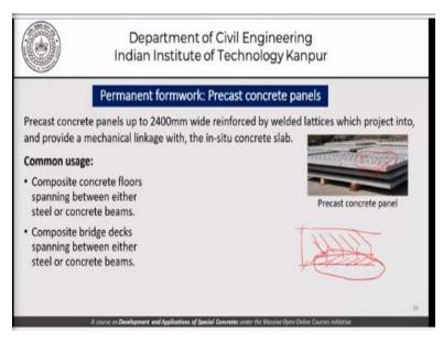
Coming to the third type of permanent formwork that we must discuss today is the precast concrete panels. So, these precast concrete panels up to 2.4 meters wide reinforced with welded lattices which projects into and provide a mechanical linkage with the in-situ concrete slab. So, what is been suggested here is that these slabs which will have a certain length and of certain width, the thickness of course is something which you can see from here.
