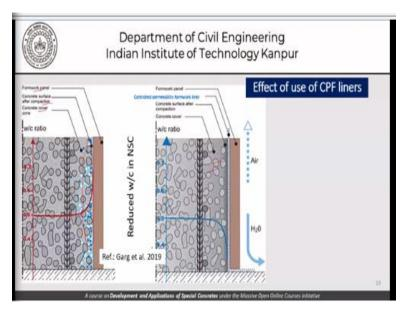
And here we are able to see again the representation of the formwork panel, the concrete surface after compaction and the concrete in the cover zone with this additional water which has been taken out leading to better quality concrete as far as the surface is concerned.
