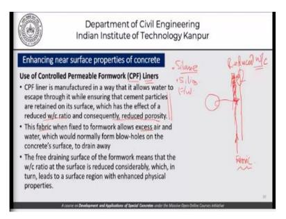
The third strategy which we can adopt to enhance the properties of near surface concretes is use of controlled permeable formwork that is the CPF liners. Now we have talked about silane applications that are an application of a product after the concrete has hardened. We have talked about microsilica which is an additive which is used at the time of construction in the main concrete itself.
