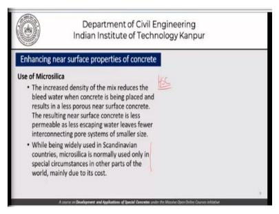
The increased density of the mix reduces the bleed water when the concrete is being placed and results in a less porous near surface concrete. The resulting near surface concrete is less permeable as less escaping water leaves fewer interconnecting pore systems of smaller sizes. So, basically what is being suggested is in this mechanism that the presence of microsilica in the concrete mix makes bleeding itself very difficult or reduces the amount of bleeding.
