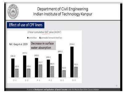
As far as the decrease in the surface water absorption is concerned, we try to carry out what is called a 2-hour cumulative ISAT test. And those of you are interested should actually look up and see how an ISAT test is carried out. And we find that regardless of the CPF liners used the values have considerably reduced, how much is the reduction, how much is the initial value of course is a matter of experimental research, so let us not bother so much about it.
