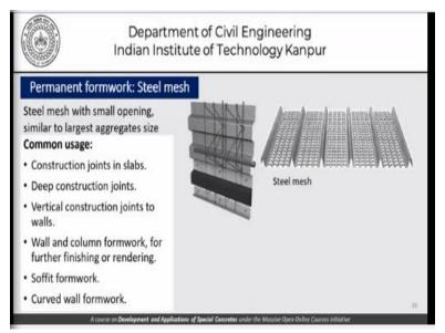
Then we have the next type of permanent formwork which is been mentioned here. That is the steel mesh, pictures are shown here for you, the steel mesh has small openings similar to the large size aggregate meshes. And they are commonly used in construction joints, in slabs, deep construction joints, vertical construction joints from walls. Wall and column formwork, for further finishing and rendering, soffit formwork, curved wall formwork.
