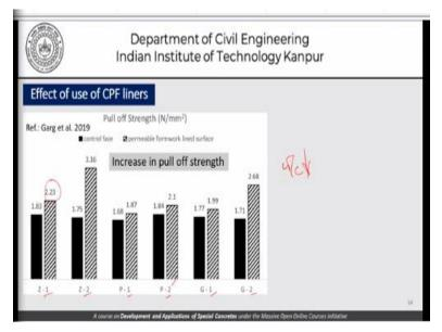
Now here are some of the results that we obtained as far as the effect of use of CPF liners is concerned. We try to do a pull off test from the surface and we found that for the different liners Z-1, Z-2, P-1, P-2 and G-1, G-2 where P is the particle board, G is the gunny bags and Z is the commercial liner. In all cases there was an improvement in the pull off strength which is basically an indication of the fact that the water cement ratio has reduced.
