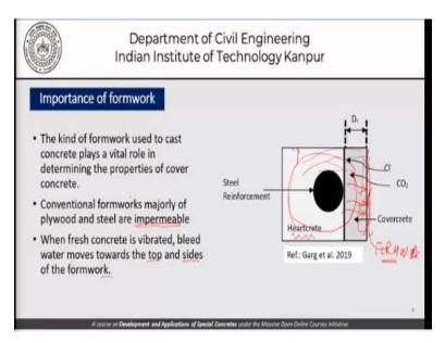
So, basically the kind of formwork used to cast the concrete plays a vital role in determining the properties of cover concrete. You will recall that as far as construction is concerned, how we do it is we put a form work here and this form work. And against this formwork we cast this entire concrete with the reinforcement of course inside it. So, the properties of this formwork are an important factor that determines the properties of cover concrete.
