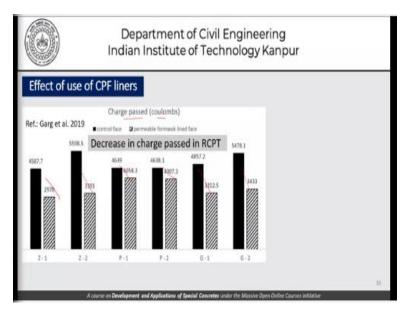
Yet another test we carried out was the RCPT or the rapid chloride permeability test where the effectiveness is measured in terms of charge passed in terms of coulombs. And we found that again the values are lower than the corresponding concretes cast without the CPF liner. Whether this is more effective than this and so on that is a matter of discussion of course which of some of these results are quite obvious.
