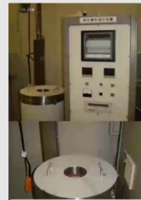
Unit for measuring temperature rise in concrete
