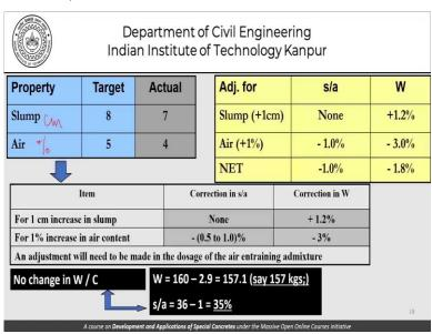
The original mix was proportioned as an entrained concrete with these numbers and the mix has to be redesigned using this does not change because that is a given the water content has been changed from 160 to 157 like I showed you before we are not changing. This s/a is becoming 35 instead of 36. Of course, there have to be an adjustment in the dosage of the air entraining at mixture to increase the air content because we got 4% whereas we want actually 5%.
