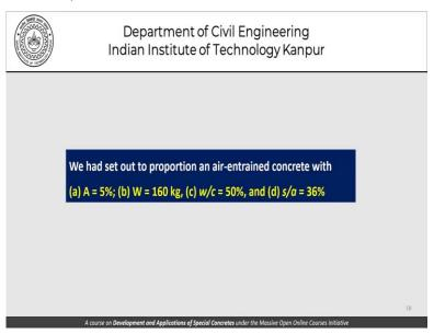
We had set out to proportion an air entrained concrete with the parameters 5% air, 160 kgs of unit water content, a water cement ratio of 50% and an s/a of 36% and with that we have determined these to be the proportions.
