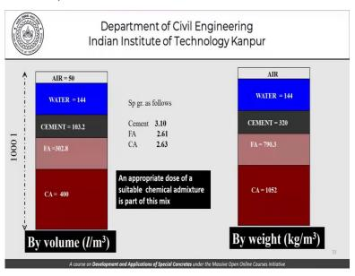
So, if we do that what we have is air is 50 litres, 144 kgs of water brings my cement content to 320 which now becomes 103.2 litres. We have this volume now to be adjusted. Now, this volume has to be adjusted but the fact is that, we are still keeping coarse aggregate to be 40%, this does not change which means that only the remaining volume will be absorbed all by the fine aggregate and this will translate to 790.
