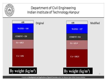
So having said that, if we do this exercise and I am not going through the details of the algebra this is what the modified mix would look like 157 kgs of water, 314 kgs of cement, water-cement ratio being 50% translating to 101.3 litres of cement, with this volume the inert material here that being proportioned using 0.35 instead of 0.36 you get 242 and 449.6 here. Use the specific gravity values to get the fine aggregate and coarse aggregate content in terms of kgs per cubic meter.
