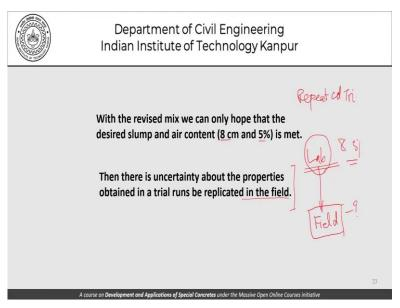
Now with the revised mix we can only hope that the desired slump and air content which is 8 centimetres and 5% is met, it may not happen and we may have to go back to the drawing board and carry out another iteration. Then there is uncertainty about the properties obtained in trial runs to be replicated in the field often times. As far as mixed design is concerned, proportioning of concrete mixes is concerned, this exercise is carried out in the lab to get a mixed proportion.
