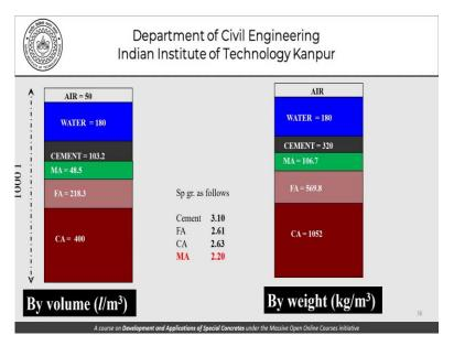
So, what we are doing here is we are keeping the water content same air is of course 5%. So, water content is 180 litres, cement we have taken to be 320 kgs brings it to about 103.2 litres replacing this 80 kgs is 106.7 kgs and given the specific gravity of the mineral admixture to be 2.2 gives me, a volume of 48.5 litres. This 400 litres does not change so the fine aggregate becomes 218.3 litres which translates to 569.8 kgs.
