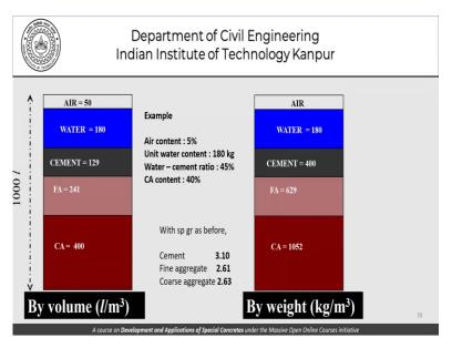
Now, obviously we start with carrying out the proportioning in a normal sense and if we do that 5% air, 180 kgs of water, 45% water-cement ratio, 40 coarse aggregate content, we get figures like this, this is by volume, this is by weight here we know 50 litres, 180 kgs i.e., 180 litres of water, 400 kgs of cement translating to 129 litres of cement and 40% here means 400 litres i.e., 1052 kgs and we have the fine aggregate to be 241 litres and 629 kgs.
