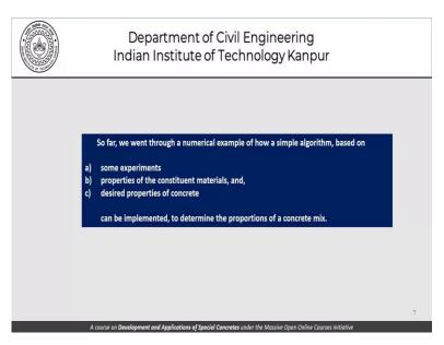
What we have done so far is that based on a simple algorithm and the principles that we have discussed. Some experiments, properties of constant materials and the desired properties of concrete, we have tried to do the determination of the proportions of a concrete mix and the exercise was largely volumetric. We went to the extent of saying that okay, we will have a 1000 litres pitcher or 1000 litres of fixed volume.
