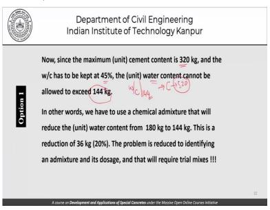
Let us examine the first route that is the chemical admixture route. What does it say that if the maximum cement content is 320 kgs? And the water cement ratio has to be kept at 45% then the maximum water content that you can have is only 144 kgs because water-cement ratio, if it is determined at 144 that will give you a cement which is 320 and that is the maximum that you can have. So, you cannot have water more than 144.
