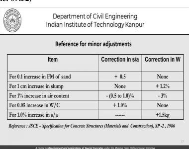
Now, here is a reference table for minor adjustments in the mix. This has been taken from the JSCE specifications for concrete structures. And, it says that if the fineness modulus of sand changes by 0.1, you need to correct the s/a that you have by +0.5. So, an increase here is a + here you do not need to adjust for water content. For each centimetre increase in slump, you do not need to correct for s/a but you need to add water to the extent of 1.2%.
