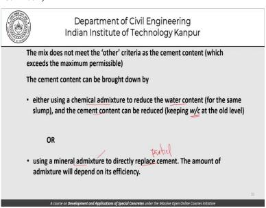
This mix does not meet the other criteria of cement content which exceeds the maximum permissible value. And this cement content can now be brought down using 2 options one is to use a chemical admixture such that the water content for the same slump can be reduced
