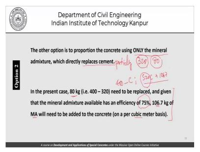
Now, let us move to the other option that we have and that is to use only the mineral admixture. We are not going to use the chemical admixture route; we are going to use the mineral admixture route and directly replace the cement partially. Of course, we only need to do it partially because 320 kgs is the cement which is still allowed and we are going to use that. So basically, what we need to do is to replace 80 kgs of cement.
