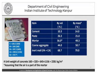
Now if we look at closely, we see that the cement is 103.2 litres, what is 160 Kgs fine aggregate, what is 247 Kgs coarse aggregate and what is 439.6 Kgs and these are the values in kgs per cubic meter. So, if we look at the relative volumes and the relative masses of these different constituents by way of percentage or in terms of percentages. We see that cement constitutes about 10% by volume and 14% by weight.
