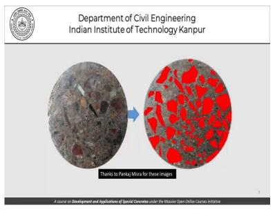
This is another picture which just shows you a real graphic picture or an image of aggregates being suspended in mortar i.e., the coarse aggregates being suspended in mortar.
