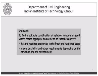
Now, as far as proportioning is concerned you have seen this slide before. The objective of this exercise is to find a suitable combination of the relative amounts of sand, water, coarse aggregate and cement. So, that the concrete has the required properties in the fresh and hardened state and meets any other requirements that the client or the codes or a particular structure might have.
