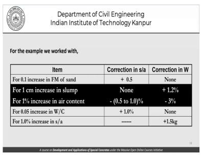
So as far as we are concerned in our particular case, we want a change in the slump value and we want a change in the air content. So how do we go about doing it, we need to do the s/a correction here and we need to do the unit water content corrections here.
