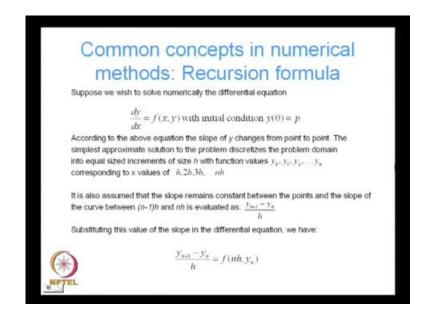
The third common numerical concept that, we wish to talk about is the idea of recursion, suppose we wish to solve numerically the differential equation d y d x is equal to f of x y
