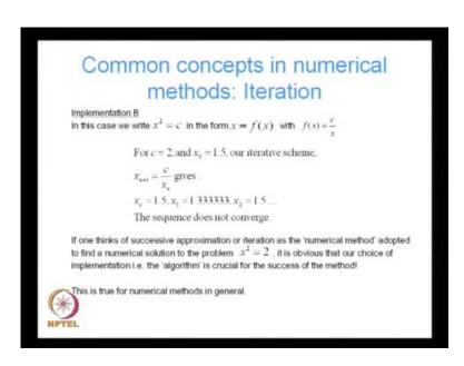
On the other hand, if we consider implementation b in which case we write f of x is equal to c by x for c is equal to 2 and x is equal to 1 point 5 are iterative scheme, which recall is x n minus 1 is equal to f of x n, which is equal to c by x n gives x 0 is equal to 1 point 5 x 1 is equal to 1 point 3 point 3 x 2 is equal to 1 point 5. So, it oscillates right the equate the sequence does not converge, If one thinks of successive approximation or
