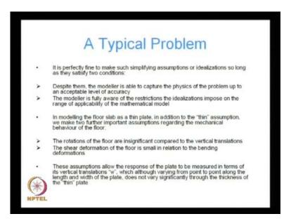
It is perfectly fine to make such simplifying assumptions or idealizations, so long as they satisfy two conditions, first despite them the modeler is able to capture, the physics of the problem up to an acceptable level of accuracy. Two, the modeler is fully aware of the restrictions, the idealizations impose on the range of applicability of the mathematical model.
