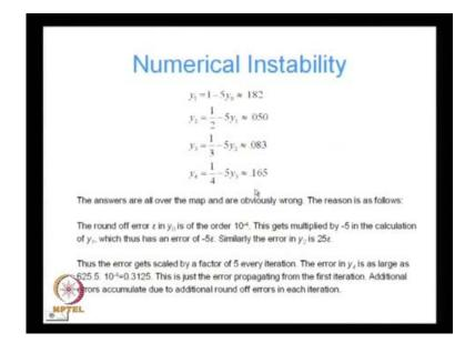
Which comes out as point 1 8 2 y 2 can be written as half 1 by 2 minus five times y 1, again according to our recursion formula, which gives me point 0 5 0, y 3 gives me 1 by 3 minus 5 times y 2 which is point 0 8 3 all being computed accurately up to three decimal places and y 4 gives me point 1 6 5. As you can see the answers are varying widely, they are all over the map and are obviously wrong, the reason is as follows.
