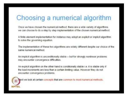
Once we have chosen a numerical method there are a wide variety of algorithms, we can choose to do a step by step implementation of the chosen numerical method. A finite element implementation for instance may adopt an explicit or implicit algorithm, to solve the governing equation. The implementation of these two algorithms are widely different, despite our choice of the same numerical method, that is the finite element method an implicit algorithm is unconditionally stable.
