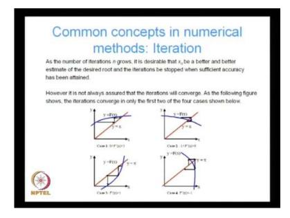
As the number of iterations n rows, it is desirable that x n be a better and better estimate of the desired root and the iterations be such stopped, when sufficient accuracy has been attained. However, it is not always assured that the iterations will converge as the following figure shows, the iterations converge in only the first two of the four cases shown below.
