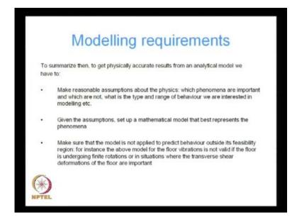
To summarize then to get physically accurate results from an analytical model, we have to one make reasonable assumptions about, the physics which phenomena are important. And which are not, what is the type and range of behavior, we are interested in modeling etcetera given the assumptions, set up a mathematical model that best represents the phenomena.
