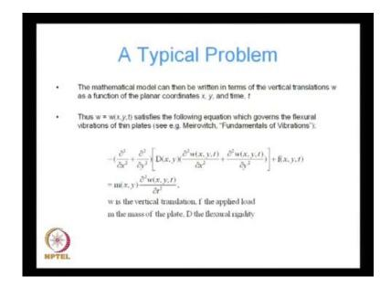
The mathematical model can then be written in terms of, the vertical translations w as a function of the planar coordinates x y and time t, thus w where w is the function of x y and t. Satisfies the following equation which governs the flexural vibrations of thin plates.
