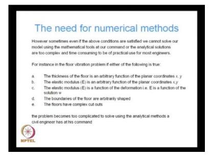
However sometimes even if the above conditions are satisfied, we cannot solve our model using the mathematical tools, at our command or the analytical solutions are too complex. And time consuming to be a practical use for most engineers, for instance in the floor vibration problem, if either of the following is true, either the thickness of the floor is an arbitrary function of the planar coordinates x and y.
