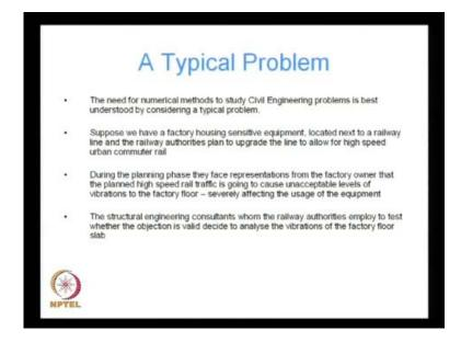
The need for numerical methods to study civil engineering problems is best understood by considering a typical problem, since I am a structural engineer I will choose a typical problem from the field of structural engineering. Suppose we have a factory housing sensitive equipment, located next to a railway line and the railway authorities plan to upgrade the line to allow for high speed urban commuter rail.
