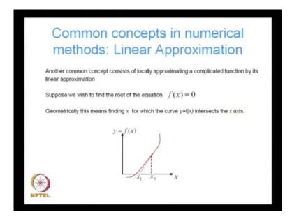
Another commonly used technique in numerical methods is linear approximation here, we locally approximate a complicated function by its linear approximation. Suppose, we wish to find the root of the equation f of x is equal to 0, geometrically this means finding x, for which the curve y is equal to f of x intersects the x axis. So, we start with the starting, case x 0 and then use a numerical method an algorithm to try to reach the solution, which is where the red curve intersects the x axis.
