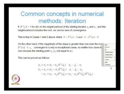
If mod f prime xi is less than 1 for all x in the neighborhood of the starting iterates x 0 and x 1 and this neighborhood includes the root, we can therefore, be sure of convergence. This is true in cases 1 and 2 above, where f prime of x is always greater than 0 and less than 1 in case of case 1 and f prime of x is greater than minus 1 and less than 0 in case of case 2, thus we can see that in case 1 and case 2 f prime of xi, the mod of f prime of xi will always be less than 1.
