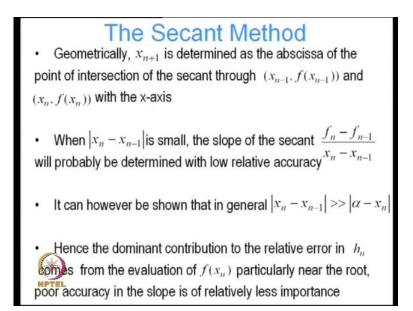
So, geometrically x n plus 1 is determined as the abscissa of the point of intersection of the secant through x n minus 1 f x n minus 1 and x n f x n with the x axis.
