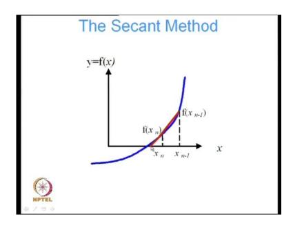
So, basically it is determined my new iterate, is determined by the point of intersection, with the x axis right of the secant right.
