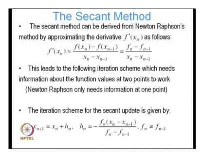
So, that is the secant method, which can be derived from Newton Raphson's method by approximating the derivative f prime x n as follows. So, f prime x n is approximately
