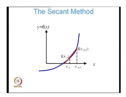
So, this is a picture I hope I have a picture of the secant method which is here, which says that earlier around in a Newton method I was actually constructing the accurate tangent here. Now, I do not construct the tangent, I see that I approximate the tangent by the secant, what is the secant it is the function value evaluated at an this point, minus the function value evaluated at that point, divided by the interval right.
