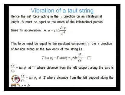
Hence, the net force acting in the y direction on an infinitesimal length d x must be equal to the mass of that infinitesimal portion times its acceleration. So, basically I am looking at this infinitesimal length of the string, and I am saying that whatever be the result of the of the tension acting on these on this little infinitesimal sample specimen that is got to result in the acceleration.
