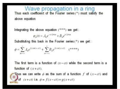
Thus each coefficient of the fourier series phi n t each coefficient, here must satisfy that equation right must satisfy that equation d 2 phi n d t square equal to minus c square 2 pi n square phi n t right. So, again to solve that equation we integrated twice right. We integrated twice and we get phi n t is equal to a n e to the power minus c t 2 pi i n plus b n e to the power c t 2 pi n right and this to integrating two times right, and I get that
