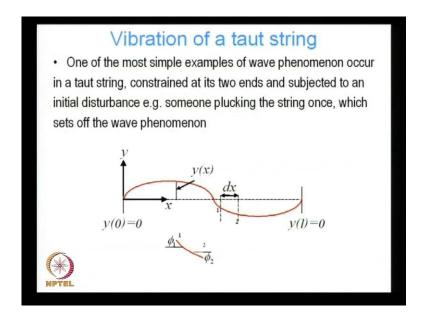
Of that specimen of that little infinitesimal length right. So, that is going to result in an acceleration and the acceleration is the rho times d x, rho times the infinitesimal length, which is the mass times the acceleration.
