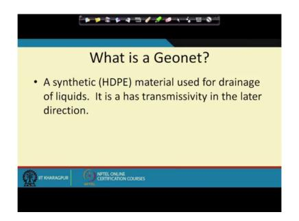
So then there is another thing used is a geo net. Geonet is a synthetic HDPE material its used for drainage of liquid and geonet.
