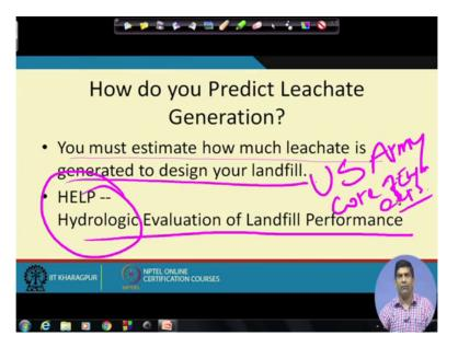
So for to get the prediction like how much the pipe is spacing as well as the pipe diameter. One of the input parameter will be what is the volume of leachate we are looking at? How much leachate is we need to manage? So in terms of how much leachate we need to manage the one thing we have to do is we have to predict because we do not know the waste how much waste will produced over 35 years period or 30 years period over the life of the landfill.
