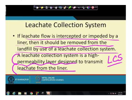
So if requirement is 2 pumps we provide 3, so even if one goes bad we will have others to take care of the work. So the leachate collection system is one since the liner in the liner system the leachate flow is intercepted. So in the liner system we have intercepting the leachate flow or impeded by the liner.
