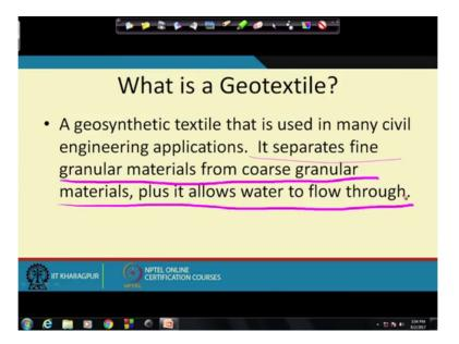
And then we have this geotextile which is a geosynthetic textile it is used in many Civil engineering application I showed you the wrapping of those pipes with this sand in between so that is the geotextile essentially as a filter. What it does it separates fine regular material from coarse granular material plus it allows the water to flow through. So basically it acts as a true filter. So that is what the geotech style does.
