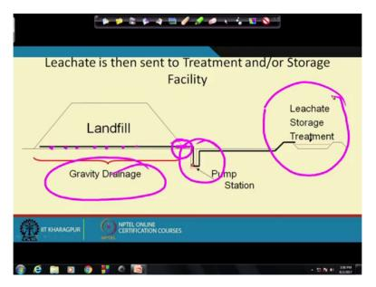
So then the leachate is then, so all those pipes that we saw those pipes are actually if it is basically those pipes are coming and joining these pipe. Let us see so these are the so the pipes are coming in and joining to these pipes over here. So those basically you will not be able to see it because it is on the other side of this pipe.
