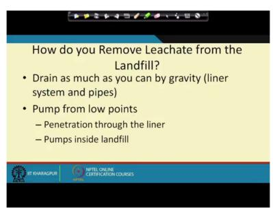
So let us talk about the leachate collection system first. So how we remove the leachate from the landfill? We try to drain as much as possible by gravity. Now we do not want to use pump inside the landfill. So for the obvious reason so we want to drain as much as possible by gravity which is the liner system and pipes. So we will have a slope we will like a slope and I will show you some pictures of that.
