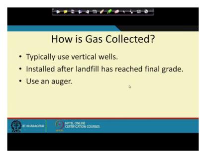
So how is the gas collected? We typically use vertical well to collect the gas, so you will have the vertical wells and we apply vacuum so we install the soft the landfill has reached a certain weight of to have reached the height and then you will use a Augr to drill the hole which also you know.
