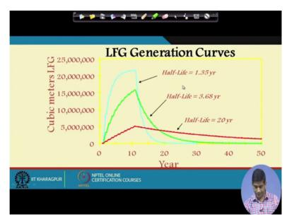
So in terms of landfill gas generation how the landfill gas will be generated over time if it is a dry tume landfill the waste is not have any recirculation going the moisture movement is not very good inside the landfill the gas production will be over a very long period of time.
