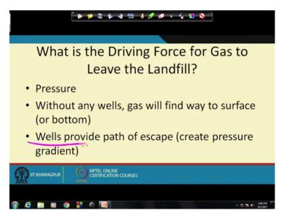
So what does the well does wells actually these gas wells provide the path of escape they create a pressure gradient so the gas travels in that particular path and gets collected. Gas collection system actually its a since most of the landfill are so huge so gas collection system efficiency is a bit low we do loose lot of gas those are called fugitive emissions. So when sometimes we have like around 65 to 70 percent gas collection is considered a very good gas
