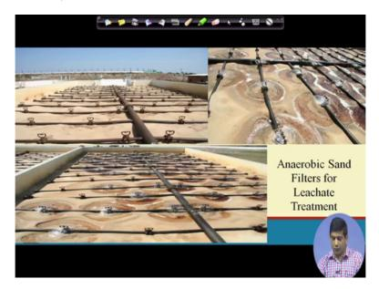
So you see a close picture of anaerobics sand filters for leachate treatment. So these are the anaerobics sand filters you see that its being aerated and at the same time it is passing through the sand filter and its moving some of this contaminates organic contaminants which is are present there.
