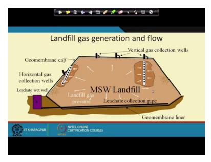
So this is a typical landfill cross section so you have these vertical gas wells. So this is your vertical gas wells similarly you have the other wells and we are looking at the cross sections so we will have several wells on top of the landfill. So that is your that is a typical like gas fill
