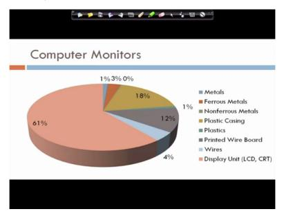
If you go to the computer monitors again we have display unit, LCD, CRT like the glass is very high and then we have some ferrous, some nonferrous and plastics, printed wire boards, wires those things are there in computer monitor.
