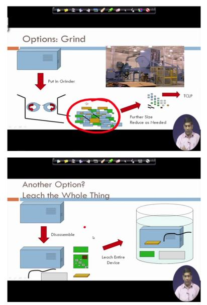
Other option is to grind it, where you can grind the sample and put it through a grinder and then you get this kind of sample after the grinding. And then you given further size reducing, so it is a further size reduce it to do the TCLP test. So then what are the another options we have, another option is you leach the whole thing.
