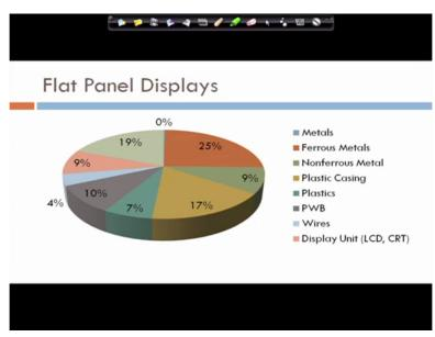
Then the flat panel display, as you can see the flat panel display unit has gone down. The percentage for display unit has gone down, we have some wire the highest that we see is the plastic again over here and metals, ferrous metals we saw that quite bit and ferrous again is coming down as well, so those things are there.
