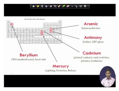
So another is your arsenic which is a toxicity concern. Antimony, cadmium, Mercury, beryllium and so these are some examples of the concerned and this is arsenic is used as a semiconductor. Antimony is used in solder and CRT glass. Cadmium it is a used for contacts and switches, plastics and batteries. Mercury we have again lighting, switching and relays. Beryllium CPU motherboard, heat sink, so those are the ones where use these elements so we need to use those elements.
