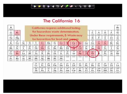
Then there is a California 16, so if you are California has additional testing for hazardous waste determination. So under this requirement e-waste may be hazardous for lead and copper, so you need to better like a check whether it is there or not so in case you have been asked to do that. So lead and copper is what we found it to be a maybe hazardous one for lead as well as for copper.
