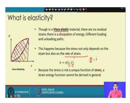
Now another instance ah for instance let us see in a see an example. This is the a material which starts if I load it its follows this path, it follows this path and when I, it follows this path and it reaches here. Now from here I remove the load and then it comes back through this path, not from the original path. What will happen?
