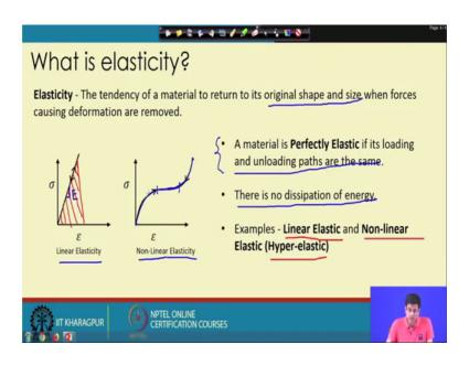
So, to start with what is the elasticity? So let us clear our concept about the elasticity. Ah I found some of us having concepts; like elasticity is where the stress is proportional to strain and all those things ah; for instance when stress ah, when I reload ah, when I load a material, when I load a sample and unload it, it comes to original position then it is called elasticity.
