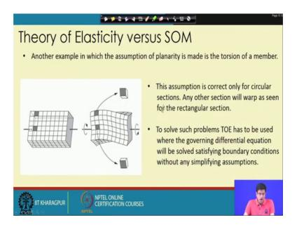
So, what is warping? So for instance if I ah, in a rectangular section ah, if I ah give a torque ; if I give a torque then there is a ah there is a change in the section ah. In the longitudinal case, if you see this carefully they will this change or different stress strain level appears. So, this kind of ah, this kind of phenomena is known as the warping. We will discuss it in detail.
