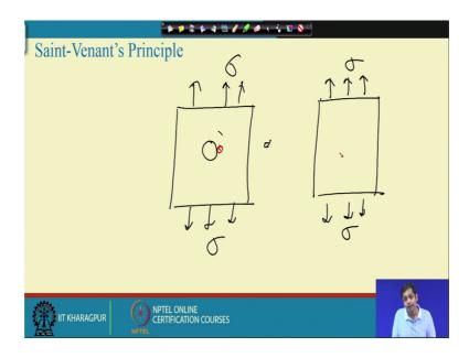
We have a plate with a central hole and which is subjected to in plane load say some say sigma; sigma. And then we will compare this we will compare this solution with a solution like this sigma and then and then sigma.
