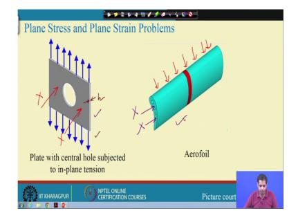
Now, some example of this for instance if you take a plate. If you take a plate and that plate is subjected to the first one. The plate is subjected to in plane loading. This is in plane tension or in plane compression whatever.
