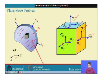
Take any arbitrary object. Suppose this is any arbitrary object whose thickness is small. This is the thickness and this thickness is h is very small ok. Now this is the x y z direction and the loads are acting all these loads say P1, P1 P 2 P 3 all these loads are acting on a plane.
