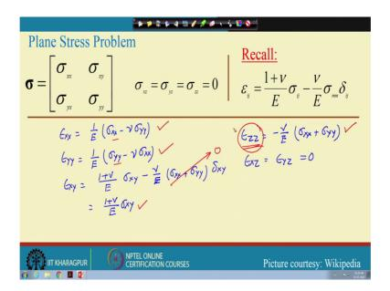
Now, for plane stress problem, we know that the stress all the components of stresses in a particular direction is 0. So, essentially your stress tensor become this. It is not a second or it is not a tensor second order tensor if you have to write it then you have to write the third column and third row as well, but they are 0 that is why it is not shown explicitly.
