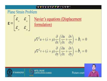
So, what you can do is, once we know what are the strain components and then stress components equilibrium equation and compatibility equation. Then we have a 3 dimensional equation general equation for stress formulation and displacement formulation. In that 3 dimensional formulation substitute the relevant only take the non 0 term and removing the term associated with 0 stresses and strain you get this reduced form.
