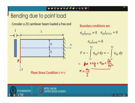
So, in this beam problem if you look carefully that we are using a 2D cantilever beam loaded at free end and this free end the resultant force is P. And we are following plane stress condition because we take c is much greater than or 2 c is essentially much greater than t. So, now, the boundary conditions as we have discussed in the last class, boundary conditions since we have following stress function based approach the boundary
