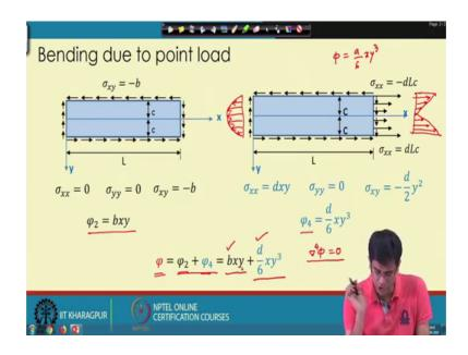
So, for instance, if you remember in the last class that we were discussing about a quadratic polynomial phi 2 of bxy which represents the pure shear case. And there is phi 4, the fourth order polynomial which is represent this stress state. So, which is essentially this sigma xx is of this form and sigma yy is 0 and sigma xy is a quadratic form or it
