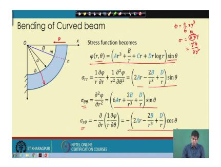
So, the stress function is are of following form. So, this stress functional is of the following form and then which is a function of r and theta the general r theta, but we have used separation of variable where this is a function of r and this is a function of theta which is the function of theta becomes sin theta. This is motivated from the bending moment equation and bending moment formula at any cross section of that beam.
