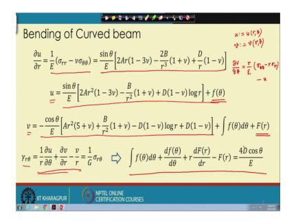
So, with this we can find out the conditions, so now the same thing we are doing here. So, here del u del r I use this and we can now after some manipulation. So, these manipulations we have not shown here so this you can just do and check this manipulation so this becomes the del u del r again similar to integrating this equation we can get the expression for u.
