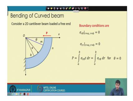
So, in the last class we were discussing about this problem where the stresses stress boundary condition using stress boundary condition we have found out the stresses. And the stress boundary conditions are those which is sigma r theta r equals to a and b equals to 0, and sigma rrr equals to a and b equals to 0 which means that along these two radial surfaces radial boundary surface there is no shear stress as well as there is no normal stress.
