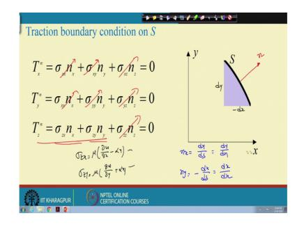
These are this is the way we derive we have the traction, and on this surface all these traction boundary all these tractions are 0.
