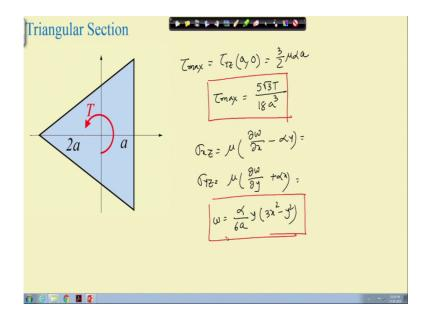
The stress will be tau max, tau max is equal to which is tau yz. You get at x is equal to a and y is equal to 0 and this will be 3 by 2 mu into alpha into a. And if you write in terms of in terms of torsion, tau max will be if you substitute alpha in the previous expression, we know the relation between alpha and T. And if we substitute this relation into this the final expression we get is 5 root 3 into torsion divided by 18 a cube ok. This is the final expression for shear stress.
