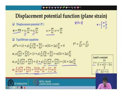
Now, here we have followed stress function approach in case of a plane stress problem and then also we can form the displacement function approach or displacement potential approach in the plane strains problem.
