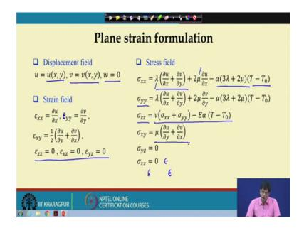
So, now this case what we can write is the displacement field. So, the displacement field I can write in terms of x and y term and then this displacement field is this u is a function of x y, v is a function of x y and w is 0. So, our usual strain field will be this so, del u del x is my epsilon x x, del v del y is epsilon y y and epsilon x y is the engineering shear strain is half of del u del y del u del v del x and this these are the plane stress assumption.
