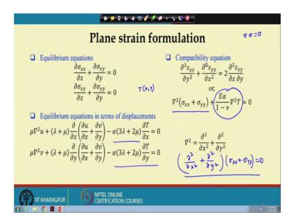
So, now in a plane strain formulation we will see the equilibrium equation. So, equilibrium equation again we know which is our basic Navier's equation of elasticity which is del dot sigma divergence of sigma equals to 0 for a static case if we do not consider the body force. So, that is del dot sigma equals to 0 if there is no body force.
