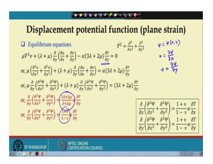
So, finally, this is the second equation, in the second equation again we can have this form so, this is. So, del t del y will be there so, that is a change and then this will be del square v. And then after some rearrangement I put the definition of psi that is I will write as u as del psi so, psi of x comma y and then del psi by del x and then v is your del psi by del y.
