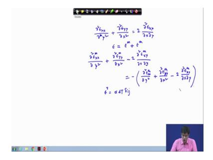
For instance, if you have this del square epsilon x x del square del y square plus del square epsilon y y by del x square equals to 2 del square epsilon x y into del x del y. Now, epsilon is actually your epsilon elastic strain or the mechanical strain and the thermal strain epsilon t h. So, I can just explain it to this in this form.
