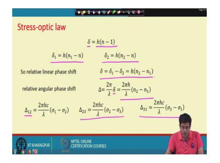
Now, once we know this we can also find out in terms of retardation. How the retardation means. So, as we know from the phase shift in a absolute air to the material if the refractive indices is, is n then the linear phase shift delta I can expressed in terms of this.
