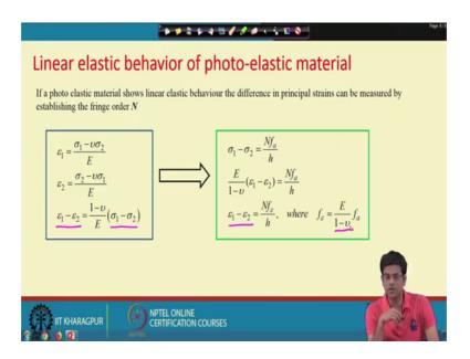
So, this is it if a photo elastic material shows linear elastic material behaviour then difference of principle strain can also be measured. So, we know from the basic elasticity relation what are the stress strain relation. So, this stress strain relations can be expressed in terms of this. So, these epsilon 1 epsilon 2 is the principal stress a principal strain and which is related with the principal stress sigma 1 and sigma 2.
