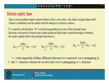
So, since a stress photo elastic material behaves like a wave plate. So, what does this mean this means that it shows a different refractive indices or essentially the propagation of light in different direction is different that means, since the refractive indices becomes different in different direction so the velocity of light essentially becomes different and then the distance travelled by the light within the medium in different direction becomes different.
