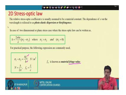
So, now in case of a 2 d plane stress problem we can just simply write it in this form. Because in a sigma 1 and sigma 2 if we take sigma 3 then this phase shift can be written as 2 pi h c by lambda and sigma 1 minus sigma 2. Now this 2 pi h c by lambda is where c the your Brewster. So, Brewster is not commonly used so what we write is that lambda by c, we define first which is known as the material fringe value.
