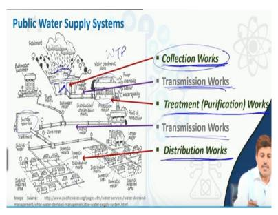
So practically as just we were discussing if we see the various components of a public water supply system, so we have the three major components of a water supply system. I am saying major components is as you can see that there is transmission work written at two stages, which are basically intermediate stages and is also quite important, but the major aspect remains that we collect water we treat purify water and then we supply water to the consumer.
