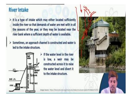
So as we discussed that, depending on this source water whether it is river or canal or reservoir or lake we may have different type of intake structures. So for the systems which are typically installed for abstracting or withdrawing water from the rivers are generally referred as river intake systems. Now this river intake is actually a system which can be located sufficiently inside the river okay or at the bank of the river.
