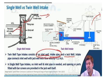
Then there are single well versus twin well intake systems. The single well intakes are the systems as just we have been discussing one single well so we will have basically water directly entering into our sump well or jack well or whatever we are providing and then from here we can pump water and send it to water works. Whereas in twin well systems, there are three components.
