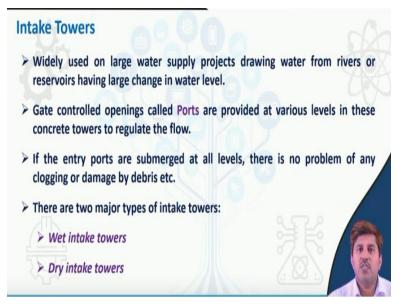
Now these were the different types based on the source, but again whether there is a water inside the intake tower or not again we can classify them as wet intake towers or dry intake towers, okay. Both of these are widely used and generally for large water supply projects from rivers or reservoirs where basically large change in water levels is often seen.
