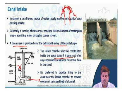
So these are some of the design criterias which one should follow while designing a river intake. Then for canal purpose, canal intakes are good for the small towns okay. Usually canals are not that big to support the water demand of larger cities, okay. So large cities usually rely either on the big rivers or lakes or groundwater systems, but for small towns canal may be a source of water supply, okay.
