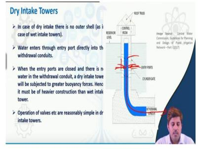
In the dry intake towers what happens that there is no outer cell. So as there is no outer cell we just have a basically concrete case and then there is a through entry ports water enter here and this eventually connects to the withdrawal conduit. So on outside it looks okay. We have water here in this and then we can have this like through entry ports and through this screens water enters directly in the withdraw conduit and then it is taken away.
