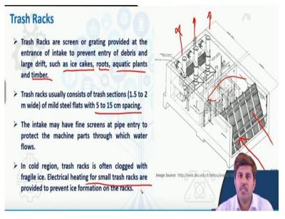
Then there are trash racks. So trash racks are generally screens and or maybe a grating provided at the entrance of the intake to prevent entry of debris in the channel. So as you can see here, from this point forwards, we are having basically pumping and other stuff over here. So pumping and these things will be done through pumps.
