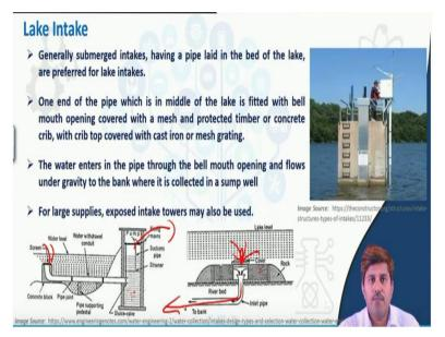
So another type is the lake intake which is generally submerged intake okay and we discussed the submerged and exposed intake in the previous lecture. Submerged intake usually will have in the lakes like we may have a pipe connecting through the lake at some places and then through a screen water enters into this pipe and then it goes to a well from where the water can be pumped and sent, okay.
