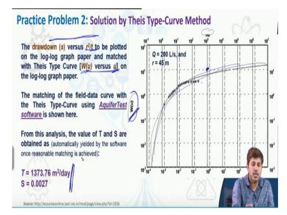
So for the Theis curve type method we know that we have standard well function curve, so 1 by u versus u W, W(u) curve we already have that and we can plot the drawdown versus r square by t curve, okay. Remember we know the drawdown, we know the r square, the distance at which the observation well is there that is r and t we know. So we can plot r square by t versus drawdown okay.
