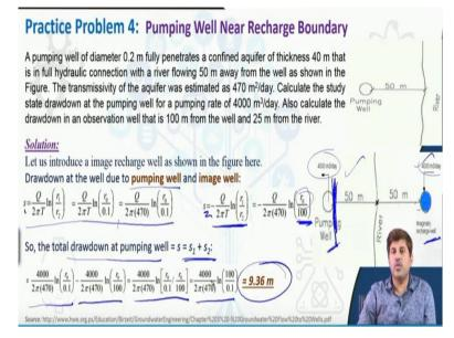
So this is another problem which is of pumping well near a recharge boundary. So we did discuss the boundary problems as well in earlier class. So it says that there is a pumping well of diameter 0.2 meter which fully penetrates a confined aquifer of thickness 40 meter, okay. So the aquifer thickness is given and it is in a full hydraulic connection with a river which is 50 meters away.
