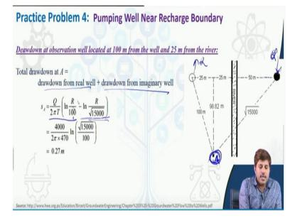
So such a well if this is our river and this is say our discharge well, okay with a flow rate of Q. This is our imaginary recharge well, without again flow rate of Q with the recharge. And we have to have an observation well which is hundred meter from the well and 25 meter from the river. So 25 meter from the river means somewhere here and then you can have a 100 meter from river.
