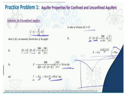
Now if we take unconfined aquifer again we can use the unconfined aquifer equation here okay. This is the typical unconfined aquifer equation. Now h 1 is 25 - 1.4 square, h 2 is 25 - 8 square 200 K ln and from here we can get the value of K. Transmissivity is K times B in unconfined aquifer. In confined aquifer we have a fixed aquifer thickness whereas in case of unconfined aquifer we do not have as such any fixed aquifer thickness.
