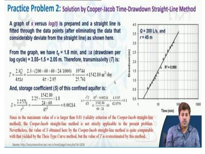
The same problem can be solved using Cooper-Jacob time-drawdown straight-line method as well. So for this we can actually plot the time versus drawdown. Now time is typically plotted on log scale. So we will have log t versus drawdown s and we will expect to get a straight line. So we will get a straight line okay remember r is 45 here and Q is 200 litres per second, okay.
