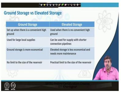
Now the difference between the Ground Storage and Elevated Storage is that Ground Storage is set up when there is a convenient high ground available, . If it is not there we should go for the elevated storage then ground storage is used for large local supplies because putting big sized elevated storage is always a challenge and is a costly affair. So that way ground storage is more economical and we can place any size of the reservoir on the ground, or below the ground.
