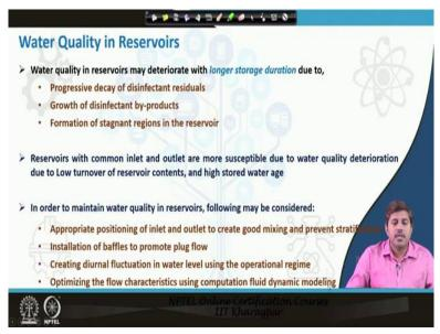
There could be various shapes there could be circular tanks rectangular sank tanks or itze tanks now when we store water in the reservoir one challenge that we see is in terms of water quality. So, water quality in these storage reservoirs may deteriorate over a period of time and generally if the storage time is longer so there are longer chances of the water quality deterioration. Now why it deteriorates so because the water which is coming into the storage reservoirs is treated water.
