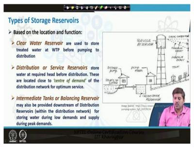
So, if we classify them based on the location and function, so there are basically three types of reservoirs, one is clear water reservoirs which are used to store treated water generally at the WTP site or just after the WTP side before it is pumped to the distribution system. So, let us say if this is our source of water this is our intake system somewhere here we have say WTP or treatment facility.
