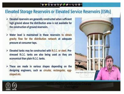
Now the elevated storage reservoirs or a limited service reservoirs as we were discussing earlier are the limited reservoirs and they will be generally constructed when there is no sufficient high ground above the distribution area is available. And if that high ground is not available then we go for the elevated reservoir. If sufficiently high ground is available then we can go for the construction of ground reservoirs.
