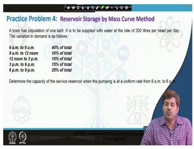
We move to the next problem which is about a town which has population of 1 lakh it has to be supplied water at a rate of 200 litres per head per day. The variations are given to us 6 to 9, 40% of the total; 9 to 12, 10% of the total; 12 to 3, 10% of the total; 3 to 6, 15% of the total; and 6 to 925% of the total. So, here even the demand is not round the clock okay demand is also distributed between just 6am to the demand is also distributed between 6 am to 9 pm.
