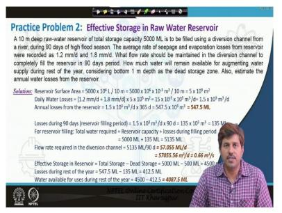
Okay, let us move to the 2nd problem. So, which is on the effective storage in the raw water reservoir. So, the question we have is 10 meter deep raw water reservoir of total storage capacity 5000 million litres is to be filled using diversion channel from a river during 90 days of high flood season. So, the important information given us is the capacity total storage capacity of the reservoir is 5,000 million litres, the depth is 10 meter and it has to be filled in 90 days period.
