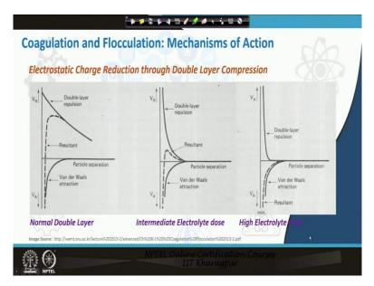
There are different mechanisms through which this destabilization and attachment of particles takes place so the coagulation and flocculation takes place. So, there are 4 major mechanisms which are considered for the coagulation and flocculation process and one of them first of them is basically the electrostatic charge reduction through double layer compression. Now we were just studying that in the normal circumstances there is a double layer form.
