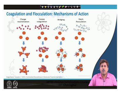
So, these are the major mechanisms for coagulation and flocculation we have charged neutralization we have sweep coagulation, we have bridging and we have kind of we may have patch flocculation kind of processes working on. So, with this will conclude this particular lecture we will talk more about the application. Now how we do these processes we have so far talked about the theory how what are the coagulation and flocculation mechanism and what is the carbonation flocculation process.
