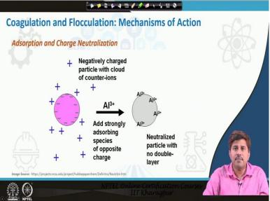
The other mechanism is the adsorption and charge neutralization. So, what happens like if say for say example we add LM doses aluminum + 3 ions we add now these are the cationic
