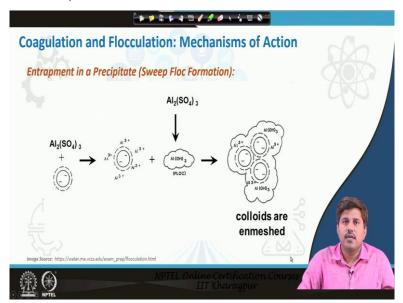
So, this is the one another mechanism which is through inter particle bridging and the last one whereas one of the most important one is the entrapment in a precipitate which is basically the sweep floc formation. So, the sweep floc formation is as such like if we are say add too much of collide particular too much of coagulant. So, these coagulant also form precipitate and a large mass of precipitate will be formed in the water.
