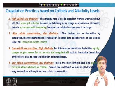
Now so based on all this we can guide on what doses must be selected or what kind of floc coagulation, coagulation flocculation system must be selected. So, if we are at high colloids and low alkalinity levels then we do not need to worry much about the pH though lower pH is better but it should not be very low. So, that it causes the it increases the solubility. So, the destabilization is generally happened by the charge neutralization because the colloid concentration is very high.
