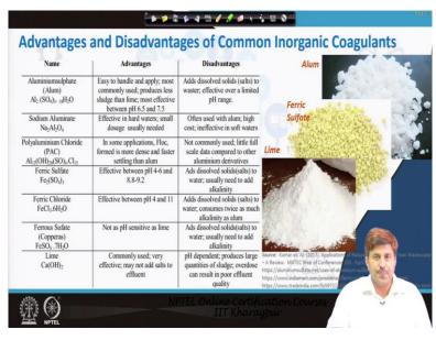
If we see the like inorganic coagulant which are more popularly more commonly used in water treatment so their comparative advantages and disadvantages like we discussed in fact these the alum which is easy to handle and apply most commonly used it produces less sludge than lime. And most effective in a range pH 6.5 to 7.5 whereas ferric chloride is very effective in pH between 4 to 11.
