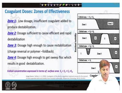
So, what typically happens under that like there are 4 different zones of effectiveness if we look at a coagulation flocculation process. So, let us say we are having a system which is having different ranges of the colloid concentrations. So, we have a chloride concentration ranging from S1 which is very low to S4 which is say substantially high colloid concentration and S2 and S3 are intermediate collide concentration.
