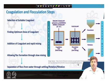
So, to begin with as we have been discussing coagulation and flocculation process, so essentially the process of coagulation and flocculation involves several steps we must need to select a suitable coagulant and then we must need to find the optimum dose of that Coagulant of course in addition we need to find the optimum operating conditions as well. And then we add that coagulant and do it in a in a flash mixture.
