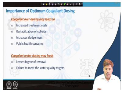
So, that is about the using Jar test you know and getting the optimum doses. The optimum dose estimation is very important because if we are adding more so like if you are going for the overdosing of the coagulant then it increases the treatment cost first because we are adding more compound more chemical it restabilizing the colloids that possibility is again there. It will increase the sludge mass because if you are adding more coagulant it is eventually going to get convert to the sludge.
