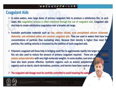
So, the label of alkalinity control of the level of alkalinity is also very essential in the coagulation flocculation process. Now that is about when we add a coagulant simply but many times what happens in basically in quite a few waters even if we add huge amount of coagulant it fails to produce the sufficient or satisfactory level of removal of the colloids. So, the flux will not be forming that great.
