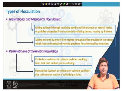
Now there are gravitational and mechanical flocculations as we were discussing. So, gravitational flocculation is when we ensure mixing by the gravity flow regime and for that purpose we provide the baffles in the basin which kind of induced the required velocity gradient for achieving flock formation. Alternatively in the mechanical systems we provide the revolving paddles with horizontal or vertical shafts or we can actually suspend paddles with horizontal oscillating beams moving up and down.
