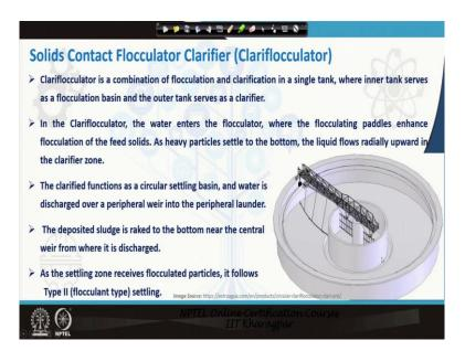
For vertical flow flocculator's it is basically like it is advisable to kind of see the energy consumption required because the head losses are likely to be higher because of the flow ugh against the gravity might be taking place. Then there are clariflocculator's which are the solid contact flocculator clarifier as we were just discussing in the beginning of this class as well that the Clariflocculator is actually a combination of the flocculation and clarification basin.
