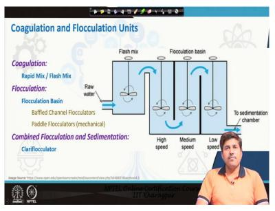
So, basically the coagulation and flocculation unit if you want to like deploy the coagulation and flocculation process in the field so what as we discussed earlier also that what we need to do is we need to select a coagulant and then we need to add that coagulant we need to kind of let the flocculation happen and then once the flocculation completes. We need to remove the floc's that are formed.
