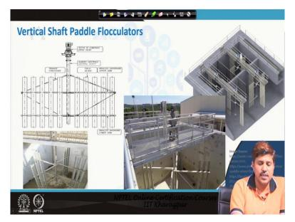
Which is which is like this so we have a vertical shaft and similarly like in the horizontal shaft we have that the shaft is horizontal and the pedals attached to this and they revolve like this. Whereas in vertical shaft the shaft is vertical and then pedals attached to that are vertical so, it would be like say this is a real basing picture so we have a word vertical shaft and then pedals attached to this and they get a rotation like this. So that way they ensure the mixing in the system.
