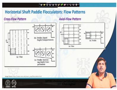
The horizontal soft-pedal flocculator can be can follow cross flow pattern or axial flow pattern ok. So, the cross flow pattern is when we have say say this is our soft say this is our soft and we have pedals attached to this. And flow is taking place in this direction, so this is a cross flow pattern because flow is taking place in this direction and the pedals rotation is the in the cross direction. So, this is the direction of say flow and this is the direction of pedal rotation.
