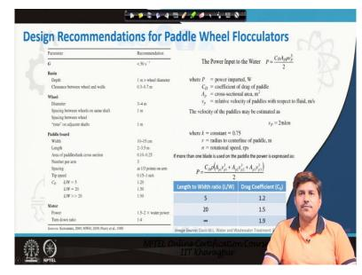
This is more important for the horizontal flow regime because in vertical flow regime we do not have any such the flow is always vertical and the movement is vertical. So, in either direction flow comes it is going to be the same but for horizontal soft-pedal flocculator this is important the cross flow one gives the better mixing as opposed to the axial flow ones. These are some of the design recommendations for paddlewheel flocculator so G value is typically taken less than 50 per second.
