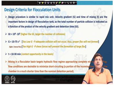
Now for designing the flocculation units the design procedure is similar to rapid mix we need to assume residence time and then based on the discharge we can actually get the volume of the tank. So, for say if we are if we are choosing 15 minutes or 20 minutes residence time so our volume will be Q whatever flow we are getting into the time whatever time we are choosing. So, this way we can determine the volume.
