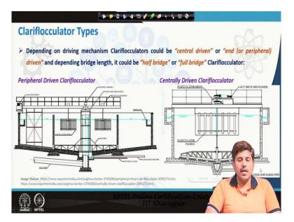
So, these are the two things which kind of decides so based on this the Clariflocculator could be central driven when we are actually like deriving it from the central so the derive mechanism is placed at the center or it could be the end driven when the derive mechanism is at the end. So, when it is at the end it actually moves through all through the periphery and when it is the center it is actually fixed at the center.
