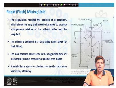
Now the rapid mix or flash mixing unit is essentially for mixing the coagulant with water so that a homogenous mixture is produced of the influent water and the chemical that we are adding. This mixing is typically achieved in a tank which is known as rapid mixer. This tank is typically known as rapid mixer or flash mixer generally because we intend to make something so we choose a shape which is which can have a good mixing which can ensure a good mixing.
