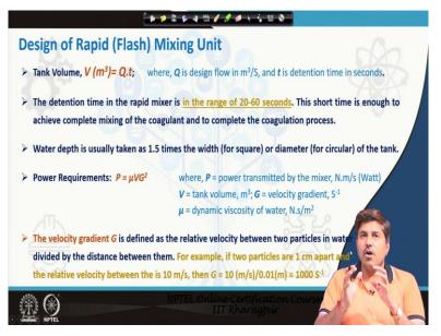
Now the point here is that the objective of a rapid mix is just mixing. So, as quickly as we can mix it would be good because our unit will be smaller. If we are mixing if you are taking say 10 minutes for mixing. So, we have to retain the flow for around 10 minutes for say and if we are say working with 1 mld flow. Let us say we are working with one mld flow. For 1 mld flow the 10 minutes would 1 mld means we are actually going to 1000 meter cubes per day.
