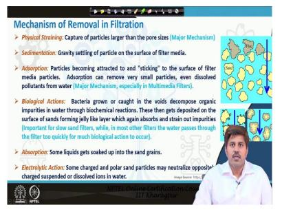
Now the removal mechanism is actually again there are multiple processes work up work on. So, the basic removal mechanism or one of the major mechanisms is the physical straining. Physically straining as in like when the water is passed through the filter media. Now if let us say we are assembling sand in a tank or in a in a chamber and then we are passing water through it so water is eventually passing through the pore spaces between the sand particles.
