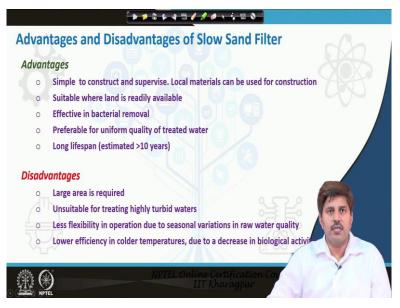
Now the major advantages and disadvantages of the slow sand filter are pretty like usual. So, the major disadvantage is that large area is required. We are working with a very low rate of filtration 0.1 or 0.2 meter as opposed to rapid sand filter which say work at 4 or 5. So, let us say like simply if you see that the area required is equal to the discharge divided by the rate of filtration. Now if our rate of filtration is 0.1 or it is 5 in case of rapid sand filter.
