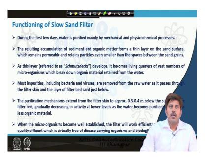
Now how this slow sand filters function so during the first few days water is purified mainly by mechanical and physical chemical processes, those process that we were just discussing so there is physical straining and adsorption which plays the major role during the first few days of the filter operation. Now as the filter keeps on working there is an accumulation of sediment and organic matter which will form a thin layer on the sand surface as just we were discussing.
