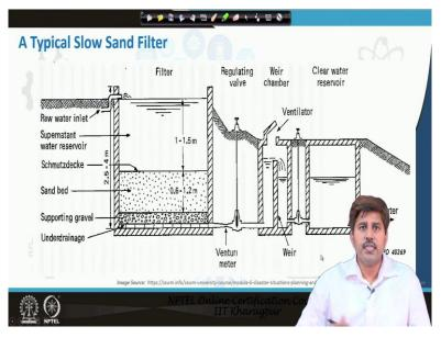
These are typical cross-section of slow sand filter again the process are same that water is put in the top then it percolates through a sand bed and then gravel supporting gravel bed and then 200 in it system it comes in a clear water chamber and from there it can be taken for further uses.
