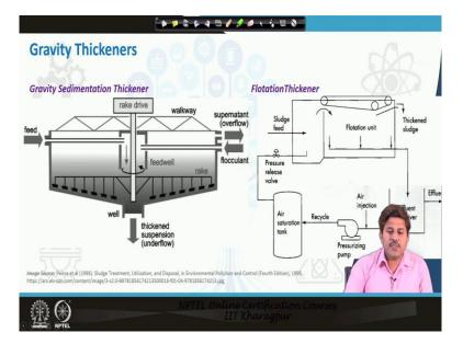
The gravity thickness are as just we were discussing it is a simple like settling basin kind of thing, so, we, we allow the feeds sludge feed to come in and then let that settle and through this crapper, we then, we can collect the thickened suspension or through under flow okay. There are floatation thicknesses which can also be considered as a gravity only because but here instead of settling at the bottom, they float at the top.
