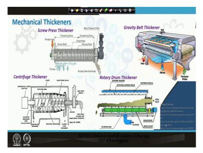
Gravity, gravity thickness are common but the like dissolved air floatation or def kind of thickness, thickness are not that common in the mechanical thickness. Again, we have the gravity belt thickener okay so there is a belt and by the force it is basically pushed through the belt, so that filtrate comes out okay and thickened sludge passes on through the belt and collected here.
