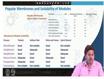
So, membrane modules and if you see like for microfiltration, ultrafiltration, nanofiltration, these different membrane models, tubular hollow fiber plate and frame spiral bone so which are good so far like reverse osmosis if you see the hollow fiber is very good okay. And this spiral bond is very good whereas these tubular and these are adequate okay. For electro dialysis tubular membranes or spiral bond membranes or hollow fibers are not suitable.
