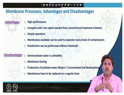
Again there are advantages and disadvantages associated with these membrane processes. The advantage is that performance is very good. They are generally compact unit so they need very less space as opposed to the conventional treatment systems. The operation is simple the membrane available can be used to kind of separate any kind of contaminant. Disinfection can also be achieved without chemical.
