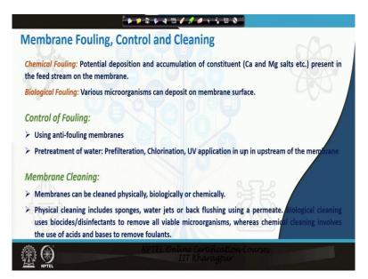
Then the membrane operation leads to the basically falling of the membrane because the contaminant is getting retained on the membrane. So, progressively there is potential deposition and accumulation of these constituents, Calcium and magnesium salts particularly if you are treating water so these present in the feed stream they will get deposited on the membrane okay.
