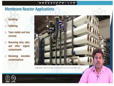
The applications of the membrane systems are for desalting, for softening purpose, for the trace metal and ion removal, removal of color order, other organic compound, removal of microbial contaminants. So, as we just discussed, RO is practically can remove any sort of contaminant okay and that is why like it is by far the most popular most safe treatment method which is usually recognized worldwide okay.
