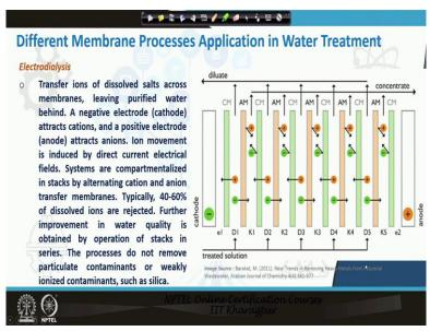
Now the electrodialysis is another type of membrane process okay so, what electro what happens in an electro dialysis, it is basically the transfer of ions that are present in the water. And how it happens let us say we are providing, we are feeding in solution here, so we are say feeding in solution here, now in this zone, we are having water present, okay. At one end we have cathode and at one end we have a node.
