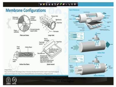
Weakly ionized contaminants like silica and those things are not removed through electro dialysis process. So, these membranes come in at different configurations okay, if you see the particularly, the like high-end RO membrane or these membranes, so there are like spiral-bound membranes so they will be bound in this and in between you have a membrane so water passes through this then permit is water is passes feed through these feed channel okay.
