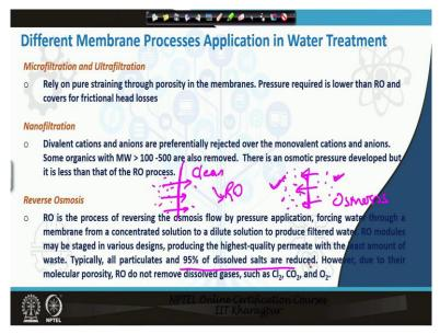
So, if you see the different membrane processes that are used in water treatment. so microfiltration and ultra filtration both rely on pure straining through porosity in the membrane. So, the like whatever the pore sizes they have the larger particles will be trapped and the water will pass through that okay. Pressure required is low because we will have just doing like pass through this.
