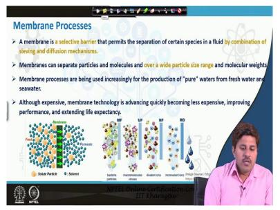
The other process which is by far considers the most advanced technology in water treatment are the membrane processes okay. These membrane processes is a selective barrier that permits the separation of certain species which basically can be either, only those compounds will not be treated which are size, which are of size finer than the membrane size, whatever membrane we are using okay.
