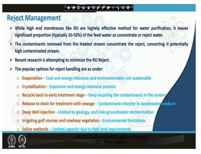
So, these are about the like falling control then the other issue is the reject that comes out of these membranes so while high end membranes like ro are highly effective for water purification. But like as we go high so they produce more reject also. The reject coming out of a nano filtration module or ultra filtration module will be much lesser as opposed to reject coming out of the RO module.
