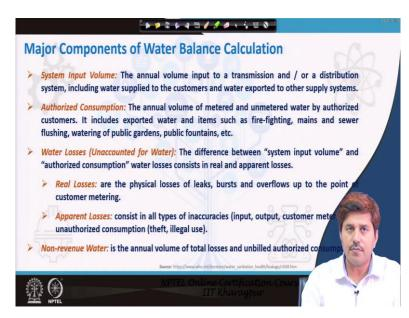
Now the major components of this water balance calculation is system input volume. So, how much water is being fed into the system. So, this is the annual volume input to a basically transmission or a distribution system it includes water supplies to the consumers and what are exported to the other supply system as well. So, if it is basically having some sort of import-export water that also needs to be included.
