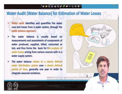
So, for the purpose of estimation of the water losses generally the water balance approach is adopted for numerical estimation. So, which is a kind of auditing the water distribution system so water audit typically identifies and quantifies the water use and losses from a water system and it is usually done through water balance approach now water audit in itself is a very broad term water audit is not only for the water distribution systems or water supply systems.
