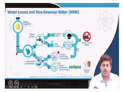
Now you know water distribution system if you see like we are actually supplying water. Now the water that are being supplied can actually be going to authorized channel or can be actually lost. So, as just we are discussing the water which is not authorized is considered as water losses. Now water losses can be apparent losses and can be real losses an authorized consumption can be built authorized consumption or unbilled authorized consumption.
