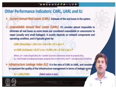
There are a couple of other performance indicators which are used which are in fact more recent. So, they are like unavoidable annual real losses and infrastructure leakage index primarily. The CRL which is current annual real losses is basically the estimate of real losses in the system. So, it is straightforward the real losses on an annual scale. Then there is an unavoidable annual real losses.
