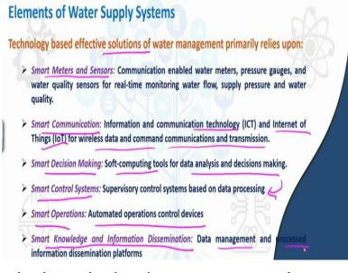
Now the elements that has to be there in a smart water supply system are basically the technology based effective solutions and these are smart meters and sensors. So these are basically the communication enabled water meters, pressure gauges water quality sensors who can real time monitor the characteristic transmitted. Transmission would be through smart communication systems.
