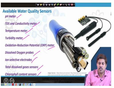
Then there are variety of water quality sensors which are available ok these water quality sensors includes a pH meters TDS and conductivity meter, there are temperature sensors, turbidity meter, oxidation reduction potential or ORP meter then dissolve oxygen probes and selective electrodes which can measure a variety of ions ok nitrate fluoride chloride ammonium so there are sensors available for variety of ions.
