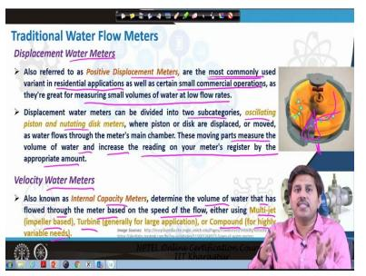
Now before talking about this smart meters let us first see what are the major measuring devices in the water supply network? So they are basically the flow meters pressure senses and some water quality parameter monitoring devices or sensors. The flow meters are traditionally either displacement type or velocity type flow meters the displacement type mostly work on a basic these are also known as the positive displacement meter.
