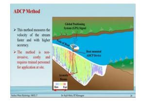
The ADCPs method measures the velocity of the stream faster and with higher accuracy. The method is non-invasive, costly, and requires trained personnel for application at the site.
