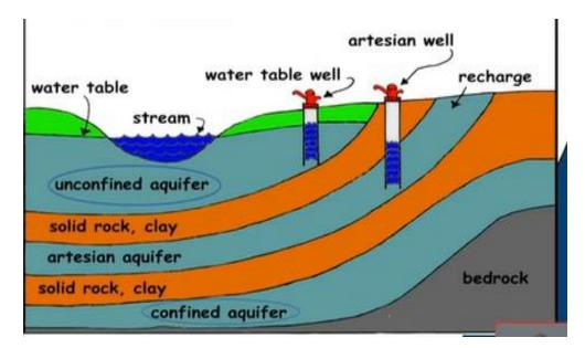
Here we can see, this is a very small sketch about the just showing you the different types of aquifers, here we can see that the unconfined aquifer. Why unconfined aquifer? Because here some rock is there lock is solid rock and this is clay solid rock means consolidated rock I have told you in the consolidated rock there are lesser chances of getting pores rather we are having the chances of getting fractures or lineaments.
