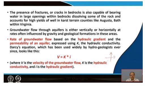
Now the presence of fractures of cracks in bed rocks because every water body is having some bedrock. And if the rocks are having some sort of fractures of cracks then what is happening is capable of bearing water in large openings within bedrocks dissolving some of the rock. So, some of the rocks are having some large openings because of the dissolving nature and account for high yields of well also, it gives the high yields of well also.
