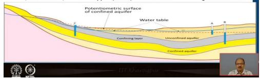
Now if you will see the diagram just below a potentiometric surface generally, we are getting in the case of confined aquifer, we are not getting in the case of unconfined aquifer. If described the total energy potentiometric surface in nothing but it describes the total energy that water is under within the confined aquifer. So, just if you will drill a well into the confined aquifer the water will rise to the level of the water table.
