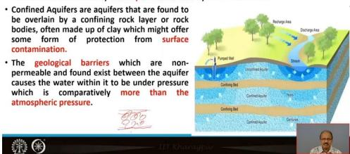
Now confined aquifer, just see confined aquifers are those as I have discussed confined aquifers are those body of water found accumulating in a permeable rock and have been closed by two impermeable rock layers of bodies. So, I have discussed in the previous slide also, if suppose any formation are there and if these formations are overlain as well as underlain by some impermeable rock's formations, rock of formations.
