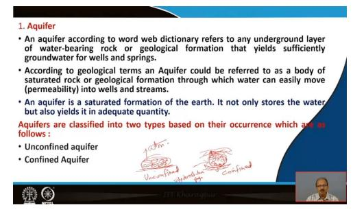
So, this is the two different types of aquifer one is the confined aquifer another is a unconfined aquifer. First of all, we should know aquifer is a rock formation, underground rock formations or water bearing rock formation or geological formation which yields sufficient amount of groundwater from for wells and springs. So, this is having sufficient amount of water. According to some geological meaning aquifer can be referred as a body of saturated rock.
