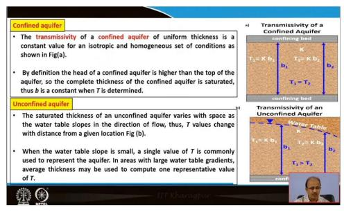
So, now the transmissivity we have discussed in greater detail, now for the confined aquifer and unconfined aquifer we will see how it is varying under two different sets of conditions. So, with this just you see right side is your diagram the transmissivity of confined aquifer this is confined aquifer. Why confined aquifer? Because this formation is having confining beds at the bottom as well as at the top.
