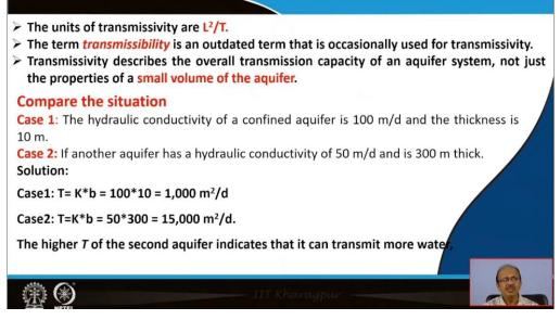
Now, we can see the unit of transmittivity are  $L^2/T$  this is the dimension  $L^2/T$  m<sup>2</sup>/s then this the unit. The term transmissibility is an outdated term that is occasionally used for transmissivity. The transmitter describes the overall transmission capacity of an aquifer system, not just the property of a small volume of the aquifer. We cannot just refer for a very small volume of water within a rock or within an aquifer.
