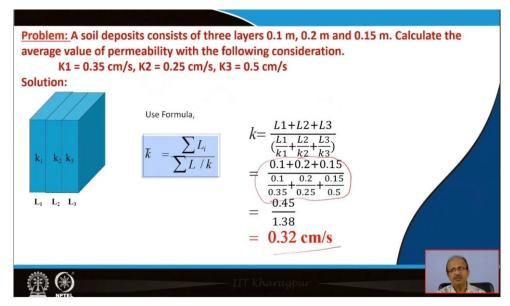
Now, on this basis we will just solve one numerical a soil deposits consist of three layers. So, now we as per the previous your description, A soil deposits consists of three layers 0.1 m, 0.2 m and 0.15 m. Calculate the average value of permeability with the following consideration. k1 = 0.35 cm/s, k2 = 0.25 cm/s, k3 = 0.5 cm/s
