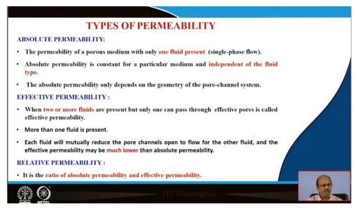
Now, in this context we can see that the different types of permeability are also there, first is the absolute permeability, the permeability of a porous medium with only fluid present. So, this is called as absolute permeability it is a constant for a particular medium and independent of the fluid type. So, it is constant for your specific type of medium and independent as per the fluid type.
