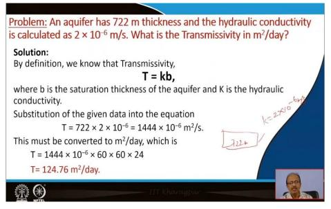
Now, just based on this, just a small numerically here that an aquifer has 722 m thickness and the hydraulic conductivity is calculated as  $2 \times 10^{-6}$  m/s. What is the Transmissivity in m<sup>2</sup>/day?.
