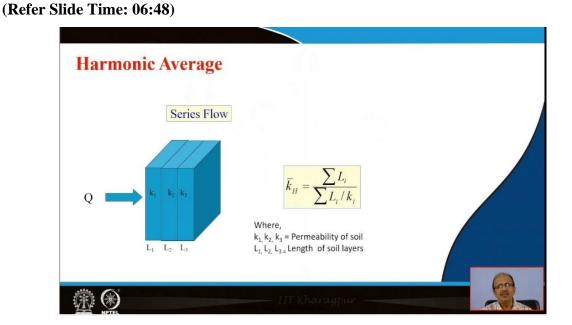
So, now next is the harmony so here, series flow we are seeing here series flow means k1, k2, k3 for three different layers of soil where L1, L2, L3 is the length of the soil layers. So, these are the length of the soil layers, in this case we are seeing that the permeability is your coefficient of permeability is the summation of L1 divided by summation of L1 by k1. So, this is the general formula for finding out the geometric and harmonic average.
