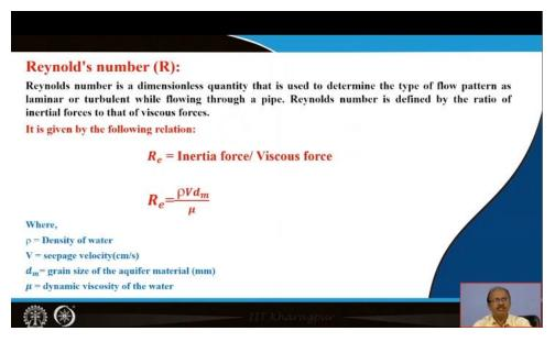
So, now the first one more thing we will just I will discuss here Reynold number. Reynold number is a dimensionless quantity which is used to determine the type of flow pattern. Which type of flow pattern is there, laminar or turbulent while flowing through a pipe. So, it is defined by the ratio of inertial forces to that of the viscous forces. Because it will the water will flow through certain pipe.
