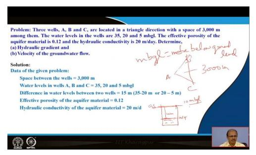
So, this is another type of Problem, three wells, A, B and C, are located in a triangle direction with a space of 3,000 m among them. The water levels in the wells are 35, 20 and 5 mbgl. The effective porosity of the aquifer material is 0.12 and the hydraulic conductivity is 20 m/day. Determine,
