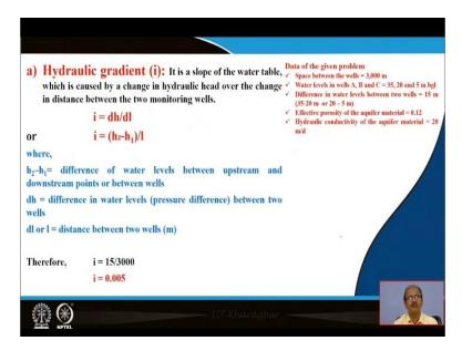
And then first question where they have to find out the hydraulic gradient of the aquifer material. So, we know we have discussed earlier also we know that hydraulic gradient is a slope of the water table which is caused by a change in the hydraulic head over the change in distance between the two monitoring wells.
