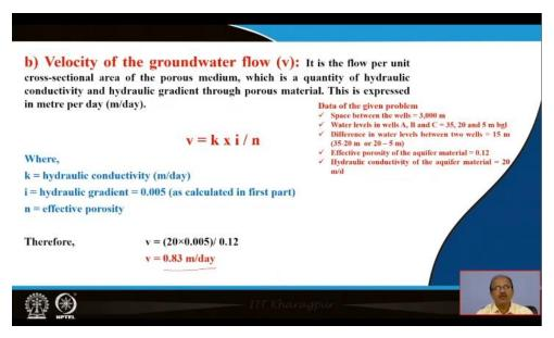
So, now we will find out the flow, velocity of the groundwater flow.
