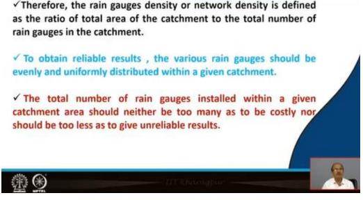
Now the rain gauge density or network density is generally defined as the ratio of total area of the catchment to the total number of rain gauges in the catchment. So, what is the total area of the catchment and what is the total number of the rain gauge in the catchment? For obtaining reliable results the various rain gauges should be evenly and formally distributed. So, this is very essential.
