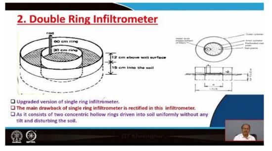
So now second is the double ring infiltrometer. So here two different rings are there you can see here also our ring is 60-centimeter ring and 30-centimeter ring and height is also given 12 centimeter above soil surface 15 centimeter into the soil and 50 centimeter is driven into the soil. It is driven into the soil and then from the earth surface to the above 12 centimeter remains and it is the upgraded portion of the single ring infiltrometer meter.
