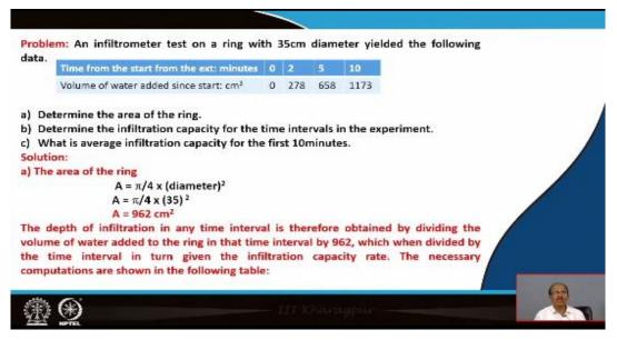
Now based on this one small numerical we can go through this small numerical An infiltrometer test on a ring with 35cm diameter yielded the following data.
