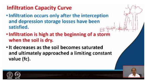
So, now infiltration capacity curve after understanding the infiltration process then the infiltration capacity. Now what is the infiltration capacity curve? So infiltration occurs only after the interception and depression storage losses have been satisfied, we have learned that time also. That when the rainfall starts, suppose that on this is the earth surface and the rainfall started drops are raised to the earth's surface.
