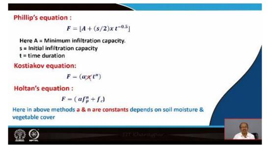
Now next equation is the Phillip's equation, in the Phillip's equation also we can find out the infiltration capacity so
