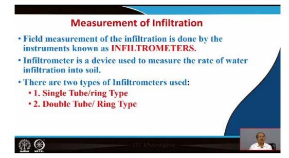
Now measurement of infiltration, how the infiltration are measured? So measurement field measurement is generally done by the infiltrometers but the problem is that the rate of water infiltrating into the soil. There are two types of infiltrometers used single tube or ring type or double tube or ring type.
