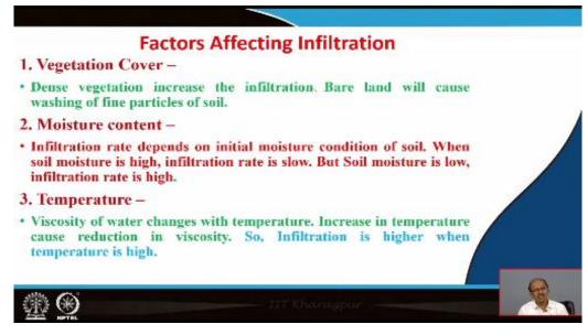
Now what are the factors affecting the infiltration capacity? This is very interesting also because we are knowing that the precipitated water will ultimately reach to the underground layer or through the soil cover only, through the land cover only. So, vegetation covers dense vegetation increase the infiltration bare land will cause washing of fine particles of soil. So, if the dense vegetation will be there it will increase the infiltration.
