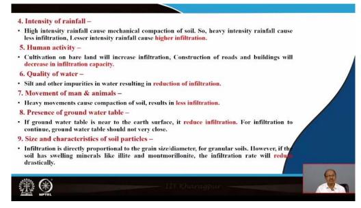
Now next is the intensity of rainfall, so high intensity rainfall causes mechanical compaction of soil because if the intensity will be more definitely the soil layer will become compact mechanically. So, once it will become compact so it will not have the pore spaces to allow water from the earth surface to inside so heavy rainfall intensity rainfall caused less infiltration. So, infiltration will be less lesser intensity and for cause higher infiltrate infiltration.
