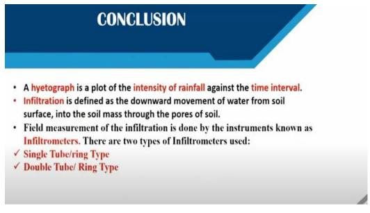
Now a hydrograph is a just a graph of the through which we can find out the intensity of rainfall against the time interval. And infiltration is defined as the downward movement of water from soil source into the soil mass through the pores of the soil. And for measurement of the infiltration is done by the instrument known as infiltrometers which are of two different types single ring infiltrometer and double ring infiltrometer.
