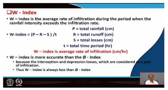
Now W-index is the average rate of infiltration during the period when the rainfall intensity exceeds the infiltration rate. So, W-index is the average the rate of infiltration. So, W-index can be written as W-index = (P - R - S) / t that P the total rainfall in centimeter, R is the total runoff in centimeter, S is the total losses in centimeter and t is the total time period in hours. So, W-index is average rate of independent infiltration in cm/hr.
