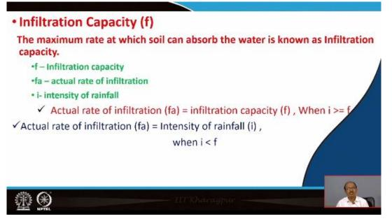
Now infiltration capacity; the maximum rate at which it is called as infiltration capacity is called as the maximum rate at which soil can absorb water is generally known as infiltration quantity. So what is the maximum rate of the soil which can absorb the amount of water is generally known as the infiltration capacity and which is denoted by fa is actual rate of infiltration.
