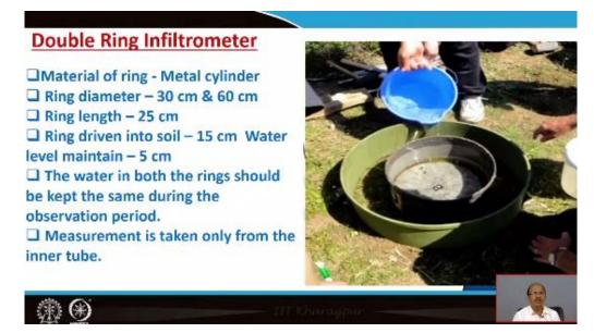
Now in this double ring infiltrometer the material of ring remains of metal cylinder, it remains metal cylinder ring diameter one is 36 centimeter other is 60 centimeter ring length is 25 centimeter ring driven into soil 15 centimeter, water level maintained into 5 centimeter then water in both the rings should be kept the same during the observational period and the measurement is taken only from the inner tube. Measurement is always taken from the inner tube, this is very important.
