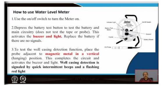
Now how to use any this water level meter because it is important first and foremost stocks is to find out the water table fluctuation. So, use the on/off switch to turn the meter and then the battery test button to test the battery and main circuitry. And generally this activates the buzzer and light, both will come from water level meter. If there are no signal just buzzer and light is not coming then you please just replace it.
