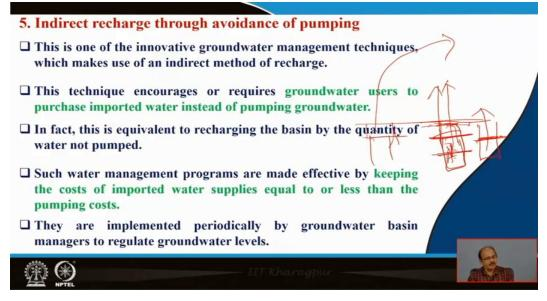
Now the next is the indirect recharge through avoidance of pumping. See what is happening in the earth's surface just what we are doing is suppose this is the earth surface and we have just beneath it is an aquifer this is an aquifer and this is the water level or this is the water level, so this is the water level of this aquifer. So, what is happening suppose if we will pump the water out then what will happen the water level will decline it will decline.
