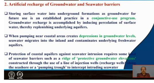
Now next it was the artificial recharge of groundwater and seawater barriers. Storing surface water into underground formations as groundwater for future use is an established practice in a conjunctive use program. So, just we are storing the surplus surface water into some any underground formation as a groundwater for future uses. So, it is actually the basis of the conjunctive use program.
