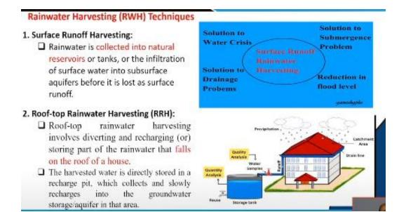
Now what are the techniques what are the techniques of the rainwater harvesting. The first is the surface runoff harvesting or at the present day it is called as your water harvesting, because here the rain water as well as surface water both are harvesting. So this rain water is collected into natural reservoirs or tanks or the infiltration of surface water into subsurface aquifers before it is lost as surface runoff.
