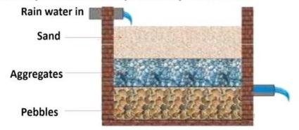
Now sand gravel filter these are commonly used filter, very commonly used filters, constructed by brick masonry and filleted by pebbles, gravel, and sand as shown in the figure. So now this is first gravel filters first filter is the sand gravel filter very commonly used filters, constructed by brick masonry you can see, these are constructed brick, this portion is considerably and pebbles, gravel, and sand are generally filled within it.
