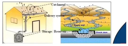
Now after this storage system now next system is the delivery system. It is the system to deliver the water for uses. So here also you can see that catchment area the room the rainwater stores here and from them this rainwater through the transportation system it is stored in the storage area system. For different uses generally a pump is being used. So that this pump can just send the water from this one and sends for different purposes it is delivered for different purposes.
