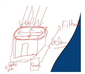
See the component of the rainwater harvesting system is basically of 6 different units. The first is the catchment area, second is the transportation, third is the first flush, fourth is the storage system, fifth is the delivery system and sixth is the filteration system. So suppose this is the roof area of any house. So the point is that this total area is the roof top area and in the roof top area if the rain will fall it will stored first at the roof top area within the roof top area.
