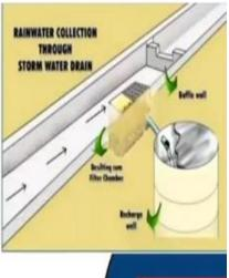
Now recharge wells for shallow water table aquifers we have learnt water table may exist at the lower depth or may remain at a deeper depth. When it remains at the shallower depth then the recharge well is best suited technique for the artificial recharging in such type of well. So, the recharges well for shallow water table aquifers up to 50 meter are cost effective because recharge can take place under Gravity flow only.
