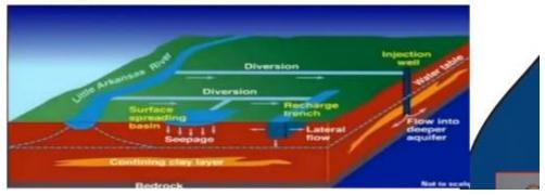
Now the subsurface method whatever we have discussed in the previous slides that were those were the different techniques of the surface method. Now the subsurface method means artificial recharge is the process but this can be done in the below the surface of the earth. So, in this method the structure lies below the surface and then it recharges the groundwater directly.
