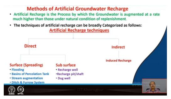
Now these methods of artificial groundwater recharge is by which the groundwater is augmented is and which is higher than those under natural condition is generally followed the 2 techniques that is direct and indirect techniques. So, direct techniques are generally divided into 2 type's surface that is spreading and subsurface. And indirect technique generally it is divided into only 1 type that is the induced recharge.
