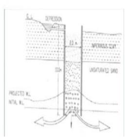
Now pitch and shafts in area where impervious layer is encountered not pervious imperviously are encountered at shallow depth the pitch and shafts are suitable structure for artificial recharge. So, in this case the pitch and shafts are the suitable structure for artificial recharge the structures are cost effective to recharge the aquifer directly the diameter of shaft should normally be more than 2 meter to accommodate more water.
