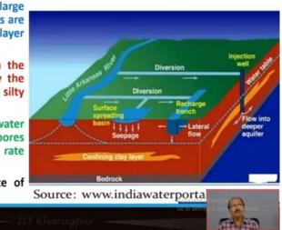
Now spreading the surface spreading this is the first method so these methods this is the first direct method so these methods are suitable with a large area of basin is unavailable. So, large area of basin is not present last area of basin is available and it aquifers are unconfined without impervious layer above it. So, surface spreading method we have seen that direct method is divided in 2 types surface spreading and subsurface spreading method.
