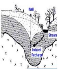
Now induced recharge it is an indirect method it is an indirect method of artificial recharge involving pumping from aquifer hydraulically connected with surface water such as perennial streams, unlined canal lakes. So, it is an indirect method of artificial recharge it involves pumping from aquifer hydraulic which is aquifer hydraulic connectivity connected with surface water such as perennial streams, unlined canal or lakes.
