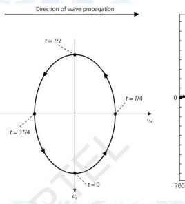
Since cos and sin are 90° out of phase, this means a particle on the surface is going through elliptical motion. Moving to greater depths, the sense of rotation changes, from counter-clockwise (retrograde), to clockwise (prograde). You can see this in the figure above, where u<sub>x</sub> becomes negative.
