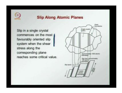
Coming back to this slide that we saw earlier, we find that in a single grain slipping and shearing will happen along the closely pack planes crystal planes with in the crystal or the grain. And, in a poly crystalline material each grain now deforms slips along different directions along the direction that is most favourably oriented as far as that crystal or grain is concerned.
