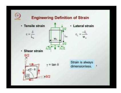
Now, we looked at stress the material when under stress under goes strain it has to respond or deform due to the applied stress and that is what we characterize in terms of strain. Tensile strain is where you have the element subjected to tensile forces tensile stresses and there is an elongation or a stretching of the material. The tensile strain is now defined as the stretch or the increase in length divided by the original L delta divided by l sub 0.
