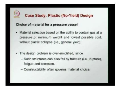
Let us, see how we can use the concept of the yield strength in design. Let us, take the case of a design of a pressure vessel which we are designing for the know yield or plastic condition. The material selection can be made based on its ability to contain gas at a pressure p. We want the lowest weight for the pressure vessel or the lowest cost possible without any plastic collapse occurring due to the pressure.
