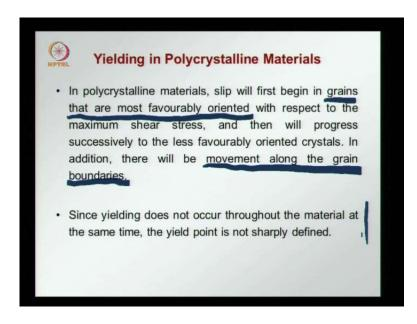
In poly crystalline materials, what we have seen? Is that slip now will occur in some grains. The grains that are most favourably oriented in terms of the stress that is the
