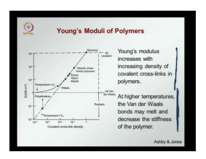
Let us, look at how young's moduli of polymers vary as a function of the micro structure, if you remember when we talked about the micro structure polymers. We said they were linear polymers and cross link to our branch polymer. And, we find that the young's modulus increases in the polymer with an increase in the density of the cross
