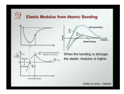
We looked at these graphs earlier. And, we saw that he can explain the elastic behaviour and a very small loads very small elongations through the condemn most diagram an the load inter atomic spacing diagram, where we saw that when we differentiate the condemn most diagram which has the energy with respect to inter particle distance or inter atomic spacing.
