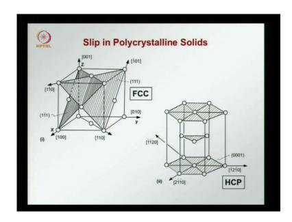
And, this is what is shown here on the left we have a material with an FCC structure with different possible slip planes covering different orientations, whereas in HCP material we have three crystal planes and all of them are along the same direction. So, a HCP material will need more stress in the poly crystalline state to be deform, and also we find that an HCP material will be less ductile less malleable than an FCC.
