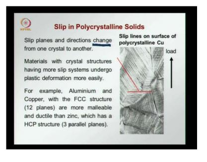
That is what we see here? In the case of say a poly crystalline. Copper given here, we have the different grains. Each of these grains has different orientation of the crystal planes. So, slipping has to change direction as even though it is loaded along one direction, we have slip changing from one crystal to the other following the crystal planes. So, slip planes and directions change from one crystal to the other.
