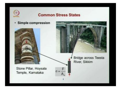
So, we have several cases, where we can identify common stress states which could be close to pure tension compression or shear. Now, in this case we see pure compression which you can have say in this example this is a stone pillar from a hoysala temple in Karnataka. Karnataka in the south of India, and we find that basically in the stone pillar you have a compressive load leading to simple compression or compressed stresses in the middle.
