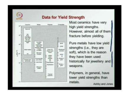
From Ashby and Jones we have taken here this diagram giving the yield strength for different types of materials. And, on the y axis the log scale we have the yield strength and different types of materials are denoted here. We find the yield strength is very high for materials such as diamond, silicon, carbide, glass and so on. Ceramics we find generally have high yield strength given by the first box.
