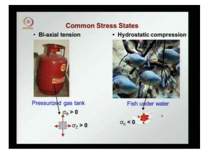
We can have other stress states which are not as simple as pure compression or pure tension. For example in the case of a pressurized gas tank or a gas cylinder, we find that the envelop of the cylinder will be under bi-axial tension. That is its being stretched in two directions they will be tension in two directions. So, you have a piece of the cylinder skin will be stretched along one direction as well as the other direction.
