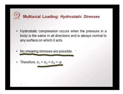
So, tau max is equal to sigma1 minus sigma 3 by 2 in the cases hydrostatic pressures when we have hydrostatic compression the pressure on the body is the same in all directions that is it is always normal to any surface an which it acts sigma 1 sigma 2 sigma 3 or all equal equal to minus p which is the pressure and therefore, no sharing is possible. So, we can we will not be able to have any shear stress when the material is a and the hydrostatic compression.
