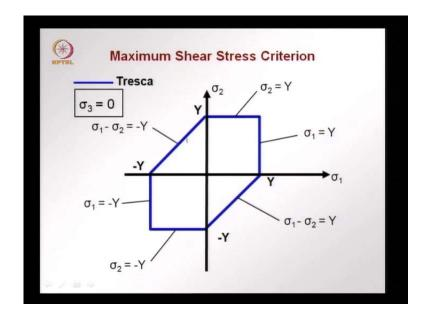
And this is represented by now by this yield surface for the tresca criterion this is a gain for sigma 3 is equals to 0 planes stress situation this surface comes from sigma 2 equals to y sigma 1 equal to y this sigma 1 minus sigma 2 equal to and so an. So, again as long as stress state is inside this yield surface failure has occur.
