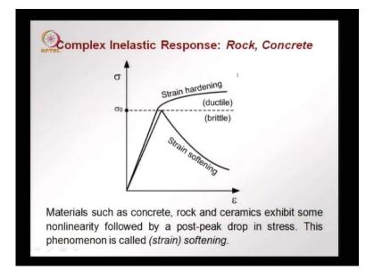
We saw in the metals when the curve goes up and it call its strain hardening this is called strain siphoning. So, any behaviour that is below a plastic Plato's brittle and is called the strain siphoning and what is above a plastic flat behaviour is called strain hardening an as I said material such as concrete rocks ceramics exhibits such type of nonlinearity there.
