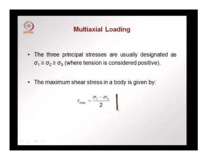
We have only axial stresses the principal stresses or usually designated sigma1 sigma 2 sigma 3 considering tension as positive sigma 1 would be the maximum principal stress sigma 3 would be the minimum principal stress the maximum shear stress in the body is given by the difference between the maximum and minimum principal stresses divided by 2.
