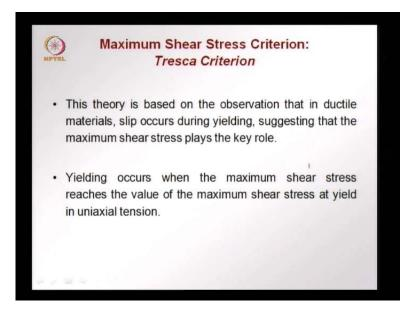
The yield surface then failure is to occur in the tresca criterion or what is called the maximum shear stress criteria we give more important to shear stress this theory is based on the observation and this we discuss extensively in previous lectures that in ductile materials slip occurs due to yielding.
