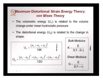
What is given a hydrostatic situation distortional energy that corresponds to the change on a distortion in the shear u v as I said this is the volumetric energy related to volume change under mean hydrostatic pressure under any arbitrary stress state they by always be a component that can be attributed to hydrostatic pressure the remaining the other part is the distortional energy is related to the change in shape.
