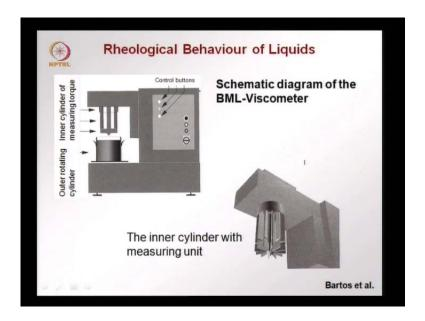
So, this is a schematic diagram of the b m l viscometer this is viscometer used in the case of in the case of concrete cement matter and. So, on where we have and outer cylinder which is filled with concrete and this rotates at a certain velocity for different velocities.
